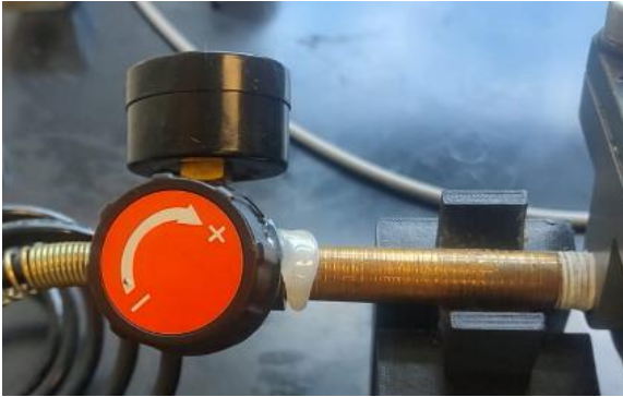
Figure 56-Flow controller on compressor and regulator
