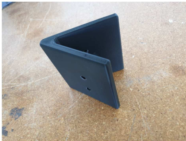
Figure 3.8: The 3D printed plate used to mount the MRR at a 45 degree angle.
