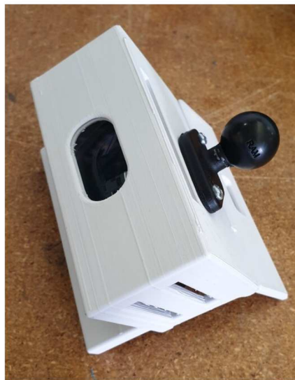
Figure 4.6: Version 2 of Housing Unit for Camera with an internal sun-glass lens and plastic cover.
