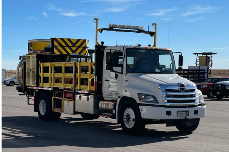
Figure 1.1: An image of the L3AV in CDOT's possession. This vehicle was integrated with a tracking array designed by CSU.
