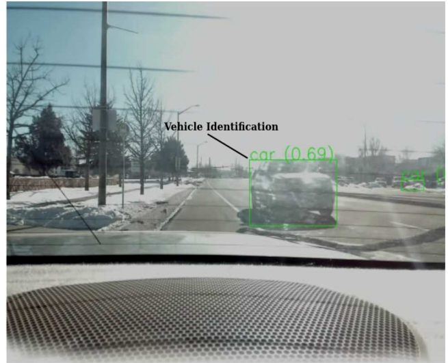
Figure 7.1: Successful vehicle tracking during stationary test, n_t=1 .
