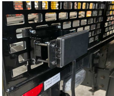
Figure 3.10: ESR mount at rear of truck
