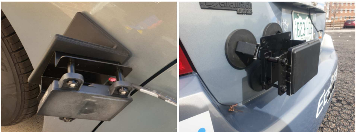
Figure 3.3: MRR radar mounted at 45 degree angle (left) and ESR mounted at the rear (right) of the 2007 Chevy Malibu.
