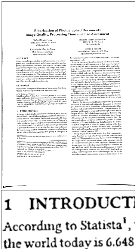
Figure 3: Top - Binarized image of an inkjet-printed document captured with a Motorola Edge 50 Pro in artificial lighting, produced by the ThreeStage algorithm. Bottom - Zoom into a part of the top image.
