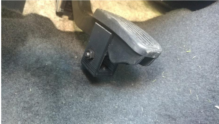
Figure 14: Installed Pedal Block on Toyota Tacoma
