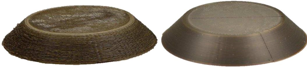
Figure 15 Preliminary ST-130 sample showing poor surface roughness on side walls and discoloration on top surface compared to a high-quality ST-130 specimen, produced later in the study.
