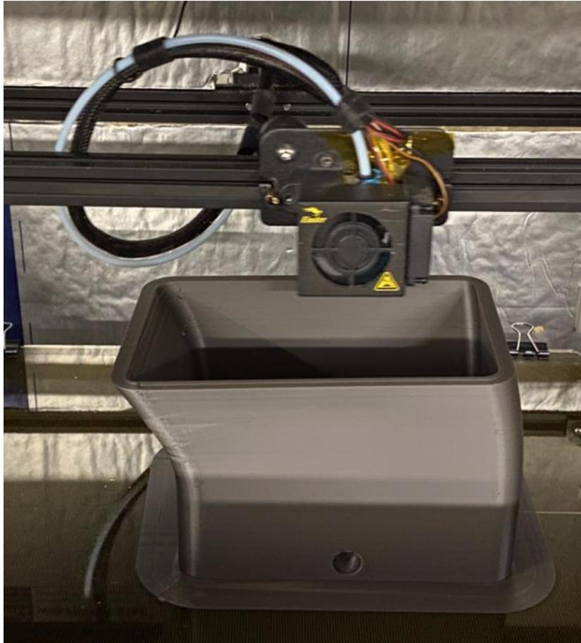
Figure 62 Hollow bent duct printing process for the Thick ST-130 Duct (2).
