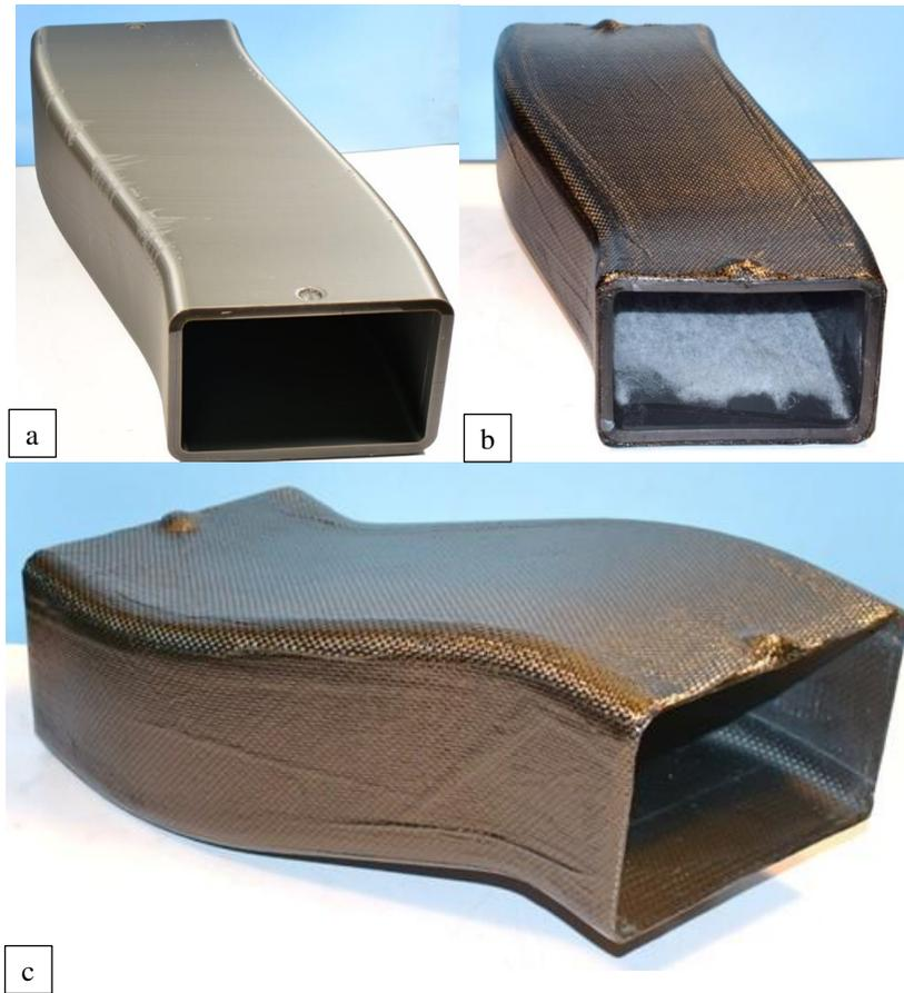
Figure 66 The printed tool (a), the composite manufactured on the tool (b), and the composite part after the tooling was removed (c).
