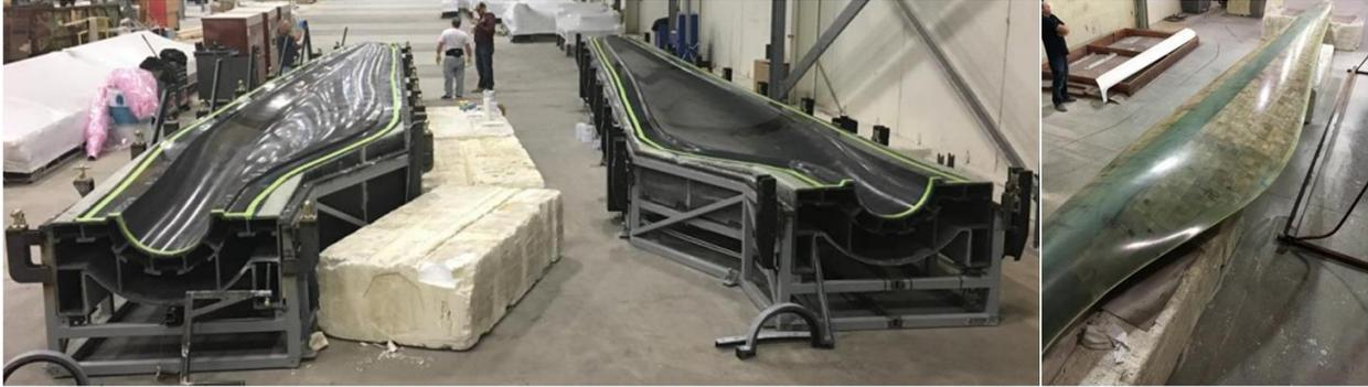
Figure 1 Two molds are used (left) for the manufacture of an AFRPC wind turbine blade (right) [2].
