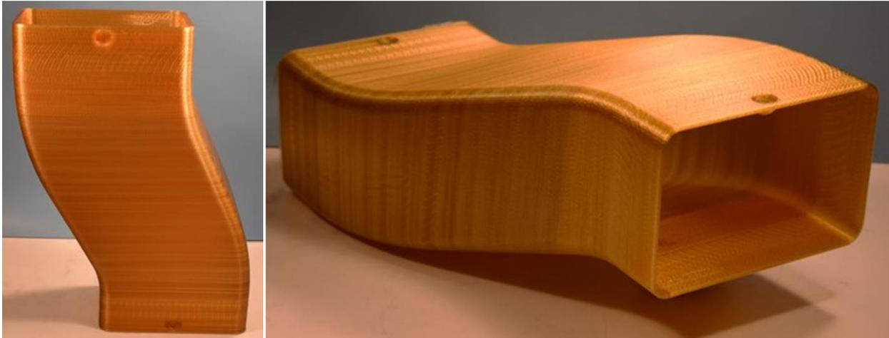
Figure 75 The manufactured tool for the Thin AQ-120 Duct (5).
