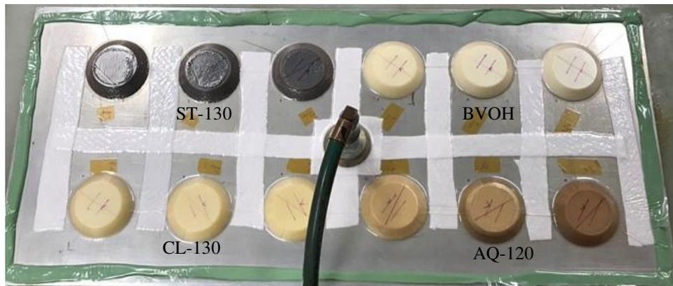
Figure 17 TPV specimens in a vacuum bag configuration prior to testing.
