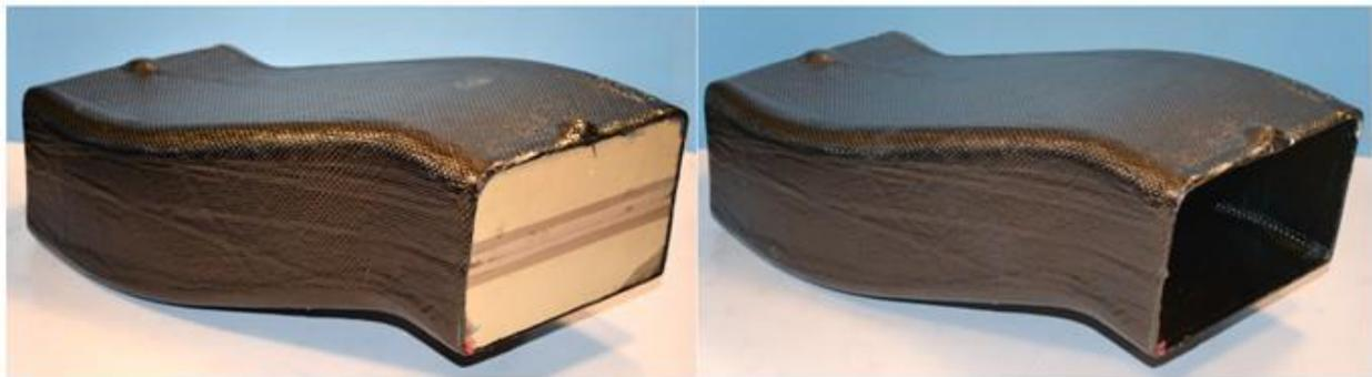
Figure 52 The completed duct before and after washout tooling material removal.
