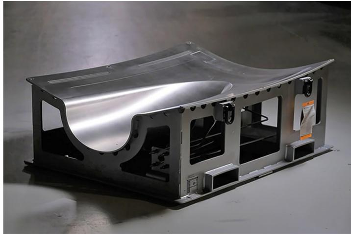
Figure 3 An egg crate structure can be seen supporting the thin critical surface of this tool [4].
