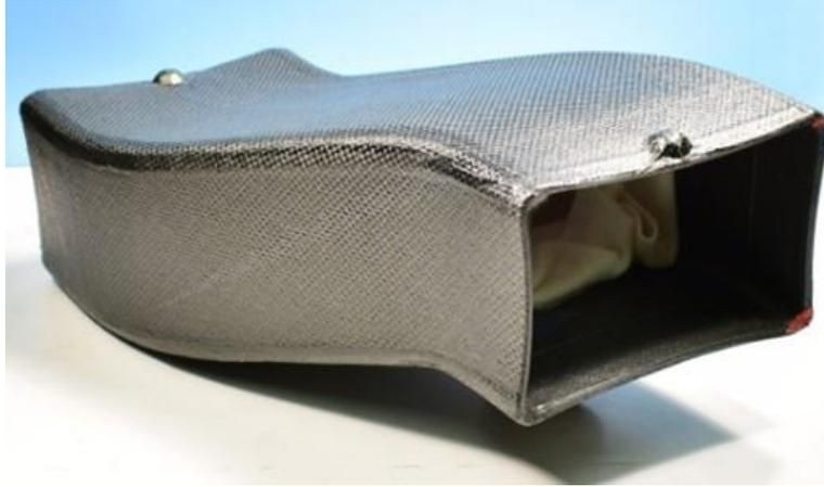
Figure 70 The cured composite with the tool left inside.
