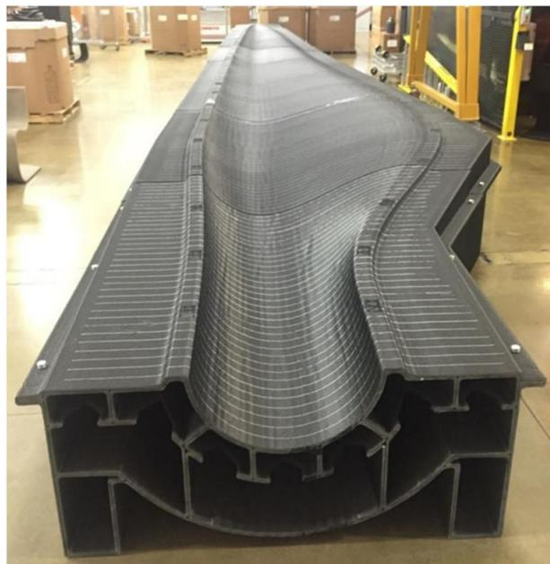
Figure 10 A 13-meter-long mold for a wind turbine blade manufactured using short carbon fiber filled thermoplastic feedstock in a melt extrusion process [2].
