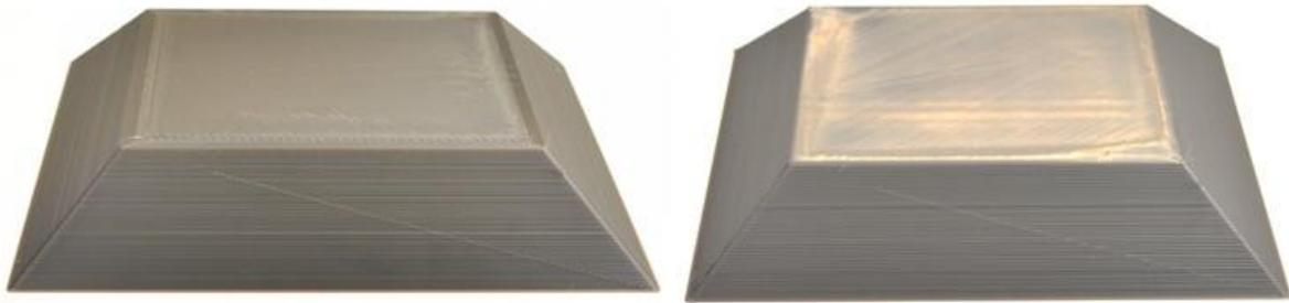
Figure 34 The as-printed Rough Pyramid tool (left) and the Smooth Pyramid tool (right).
