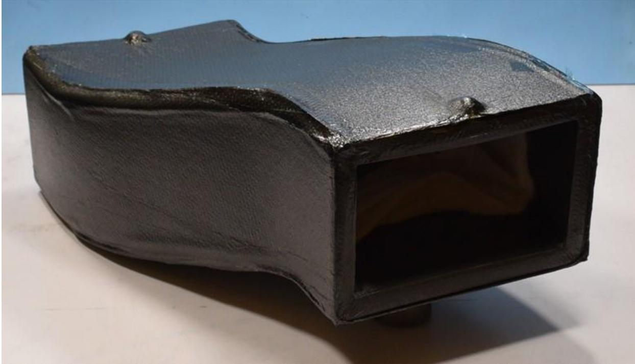
Figure 83 The composite cured on the Extra Thick ST-130 Tool 7.
