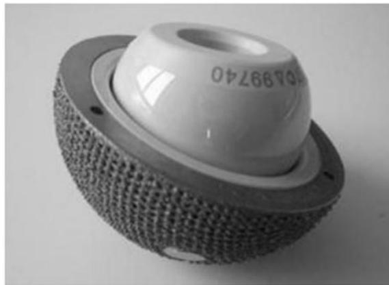
Figure 7 Acetabular cup produced using a powder bed fusion process [24].
