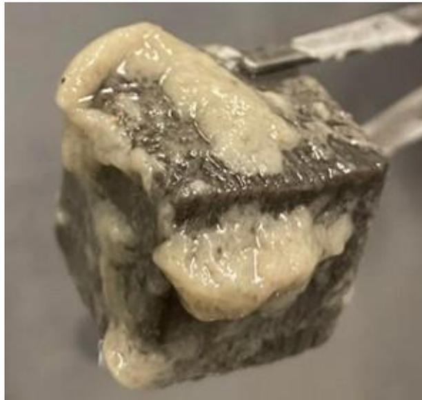
Figure 29 The gel-like substance forming on the surface of the ST-130 sample during dissolution trials.
