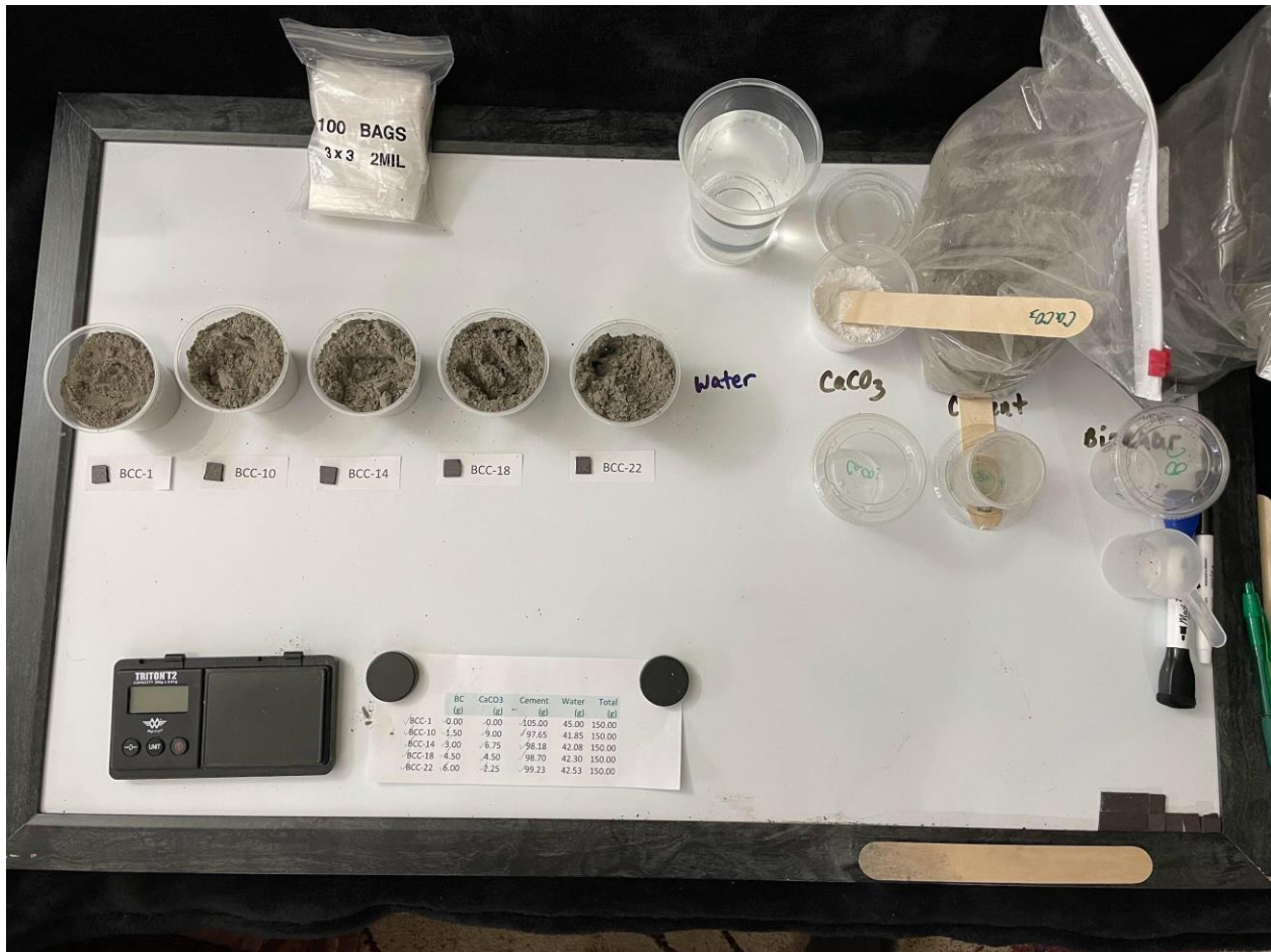
Figure 6. Validation of workability using the lowest water-to-composite (WC) ratio of 0.3 with other components of various amounts from BCC-1 (control), 10, 14, 18, and 22. Workability was confirmed in each. The lowest water-to-composite ratio was chosen since all mixtures would have greater workability than these.
