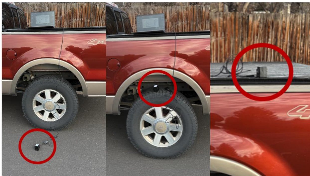
Figure 3. OPC-N3 at Ground Level, 3-feet, and 5-feet
