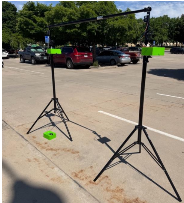
Figure 5. Roadside Infrastructure with Sensors on Top of Green Boxes
