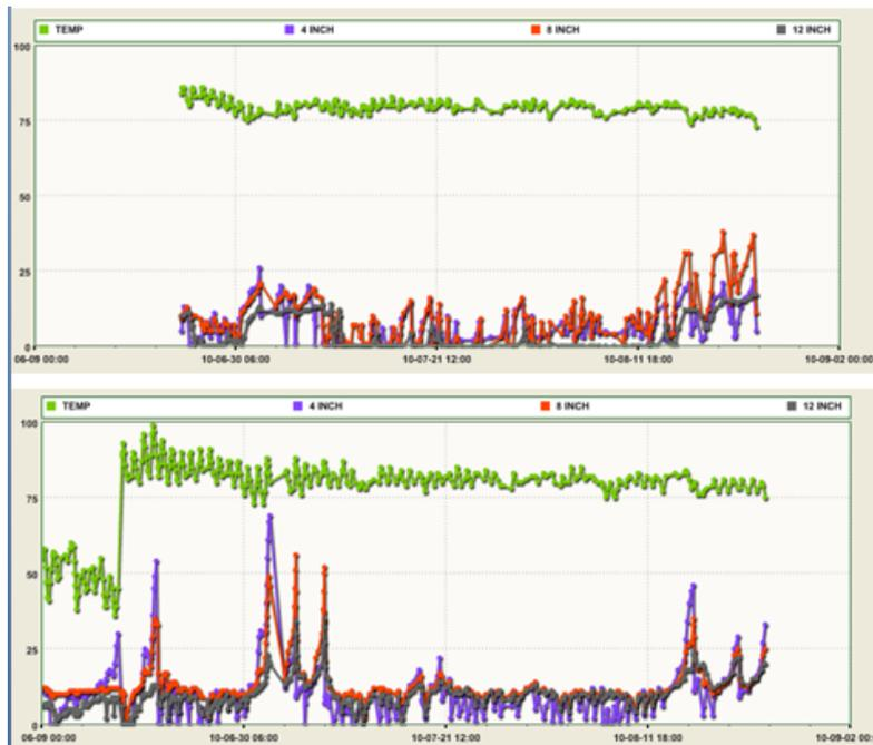
The top set of data is an area with clay loam soil that received 60% of the base application depth.
