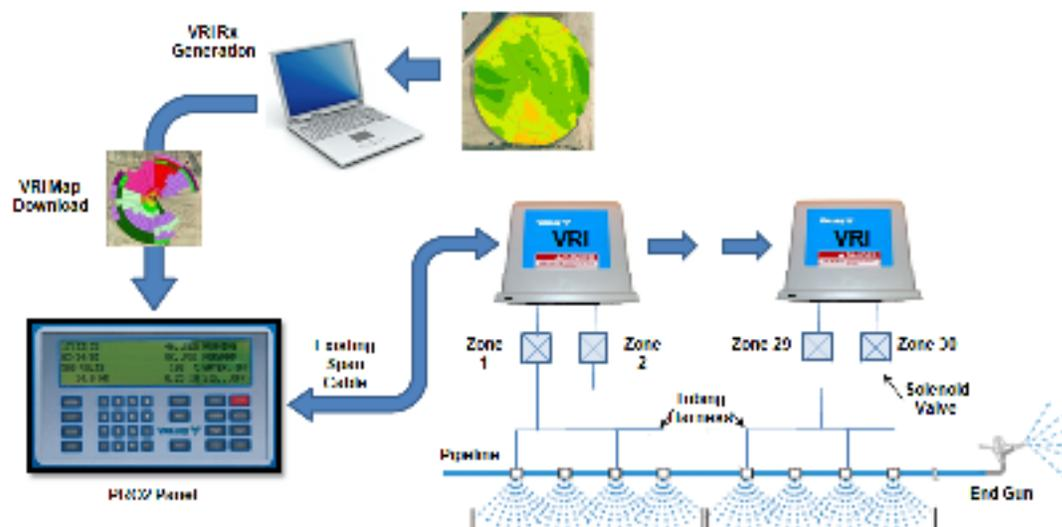
A prescription that is specific for the field is created with the VRI Prescription Software, which resides on an external computer. The prescription is then loaded into the Pro2 control panel. The VRI Prescription Software allows prescriptions to have up to 180 sectors around the field, each sector as small as two degrees.
