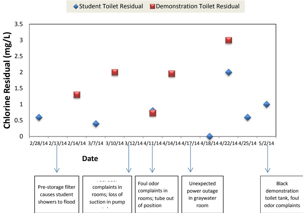
**Figure 6.4 Chlorine Residual Concentration Measurements in Demonstration Toilet and Student Toilets**
