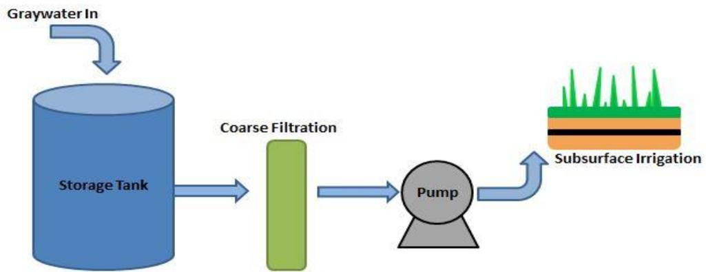
Figure 2: General Process Schematic for Graywater Subsurface Irrigation
