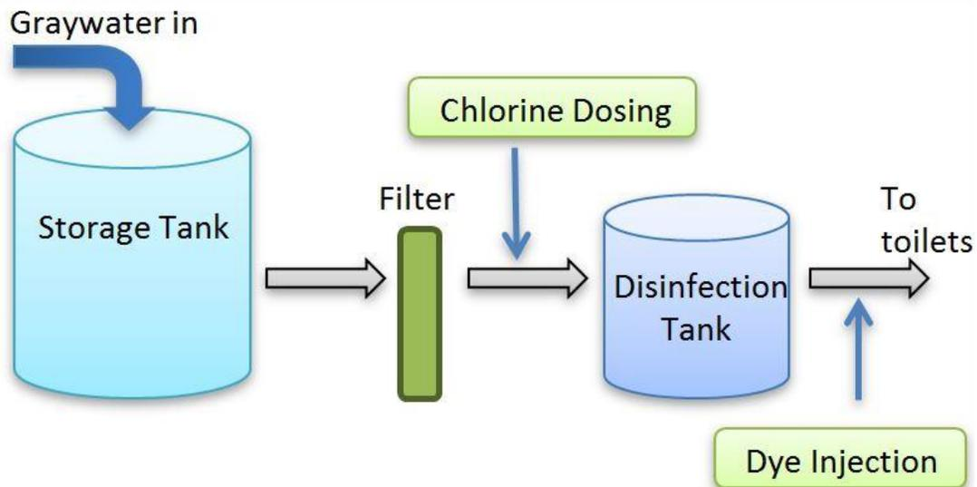
**Figure 6.1 Graywater Treatment Process Schematic**
