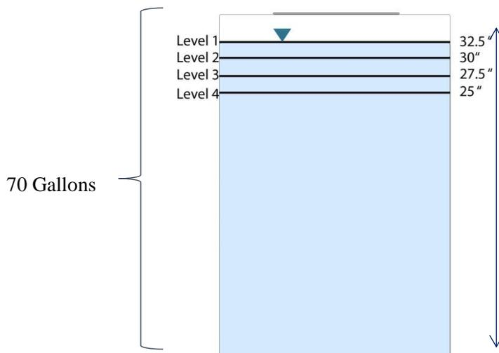
**Figure 6.3 Ultrasonic level sensor design. (Adapted from Hodgson, 2012.)**
