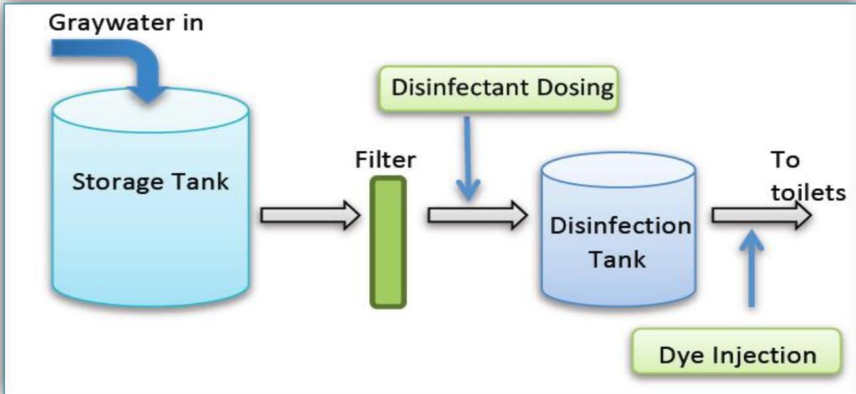
Figure 2: Graywater Treatment System Schematic
