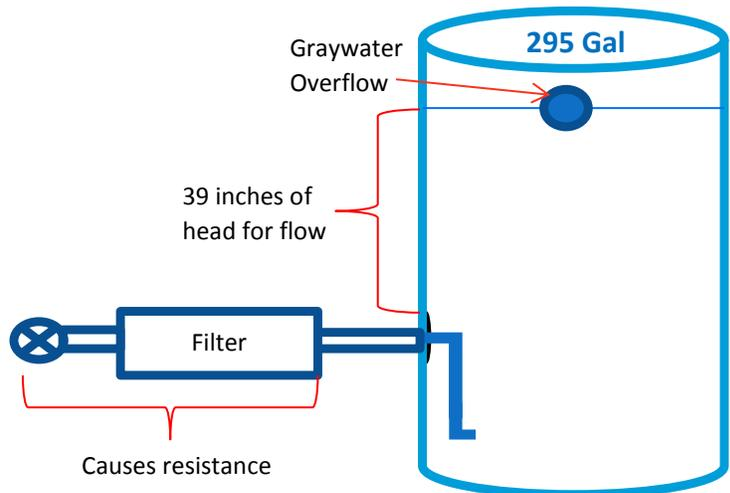
**Figure 6.5 Schematic of Head Requirements in Graywater Storage Tank.**
