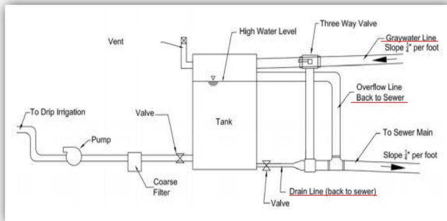
Figure 4: Graywater tank components (Bergdolt, 2011 URL: [Link](#))
