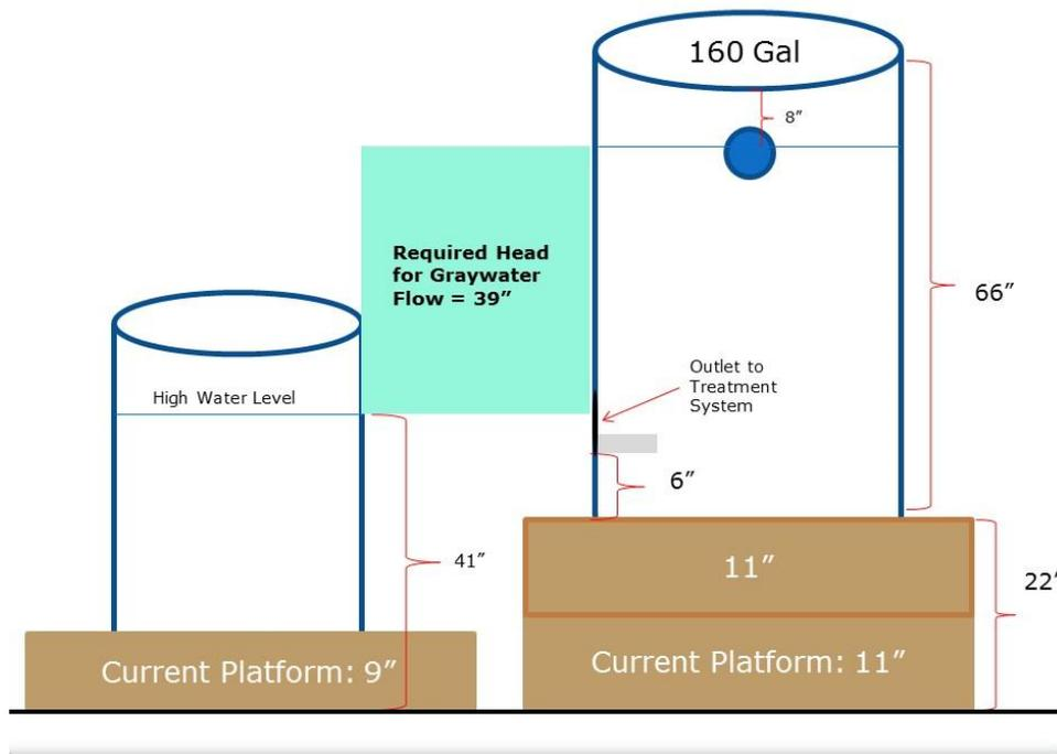
Figure 6.15 Schematic of Proposed Graywater Storage Tank Design
