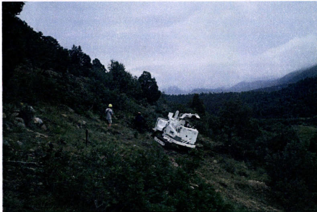
Echo Hills, Tracked Chipper on 50% slope
