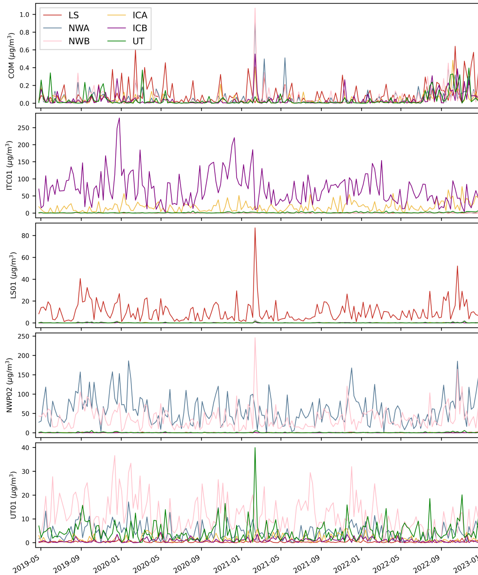
Figure C.1: AERMOD simulated weekly plume concentrations at five monitoring sites (COM, ITC01, LS01, NWP02, and UT01) from six O&G well pads (LS, NWA, NWB, ICA, ICA, and ICB) with unit emission rate of 1 g/s, respectively.
