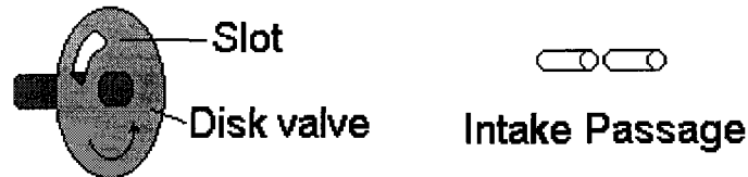
Figure B4 The disk valve with slot and air passage shown apart.
