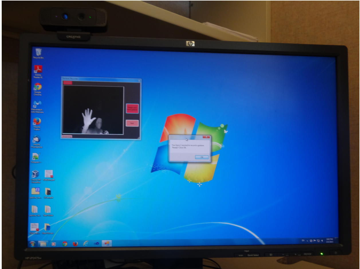
FIGURE 3.1. The PersoSys setup. Using the Intel SDK camera, PersoSys enables users to define hand gestures for tasks.
