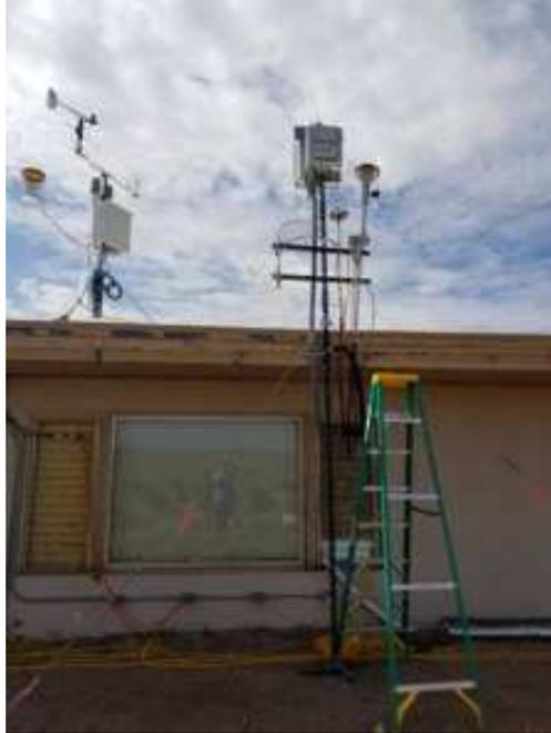
**Figure 2.1:** Instrument inlets are shown above the CAVE Biology Office. Instruments sample from approximately 6 meters above ground level.
