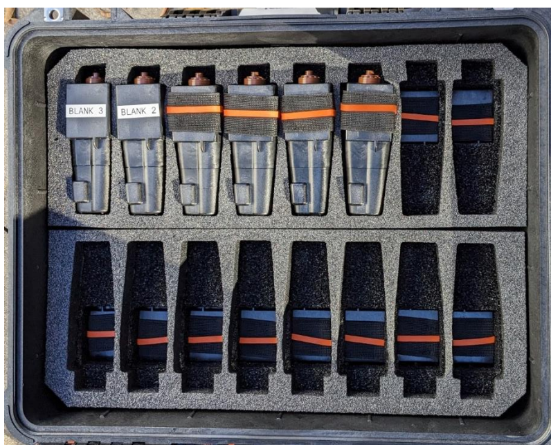
Figure B9: Ready-to-use AirPens in a hard case. Samplers were stored in this setup overnight before the deployment.
