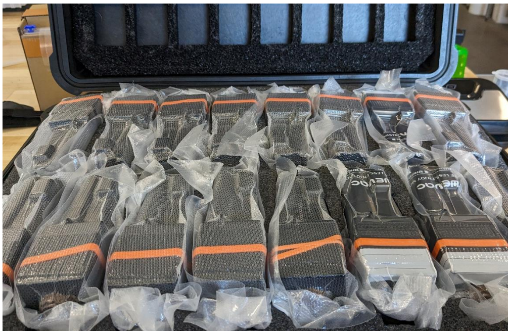
Figure B7: “Ready-to-use” AirPens vacuum sealed individually and packed in a hard case with foam dividers. Samplers were shipped in this setup from the laboratory to the field.
