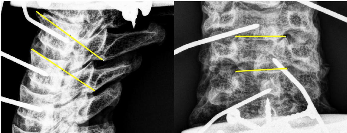
Figure 55: (Left) Intervertebral angles were measured in flexion and extension by comparing the angles made between the yellow lines at  $\pm 0.75$  Nm. These lines were drawn between the anterior/caudal endplate and the posterior/cranial wall of the spinal canal. (Right) A similar procedure was used to measure intervertebral angles in lateral bending. These lines were drawn between the uncinat processes.
