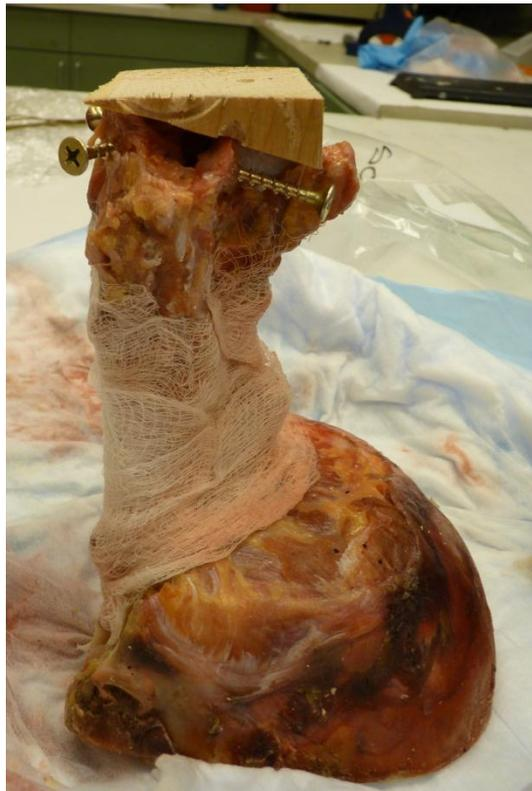
Figure 24: A wooden wedge was affixed to the caudal face of C7 to maintain a physiologic lordosis angle when potted in PMMA.
