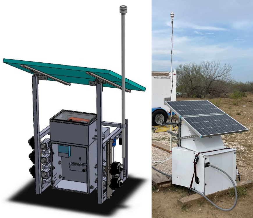
Figure 3.1: The controlled release rig (Left side shows the conceptual CAD model, Right side shows the completed device in use during testing).
