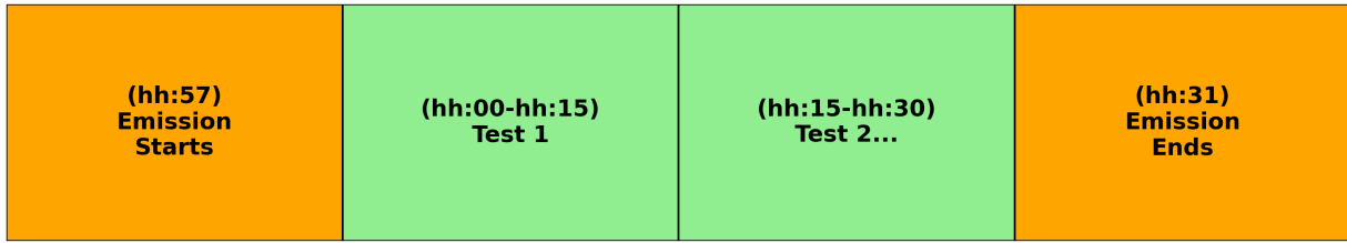
Figure 3.3: "Test" definition in relation to 15 minutes reporting intervals based on the defined protocol.
