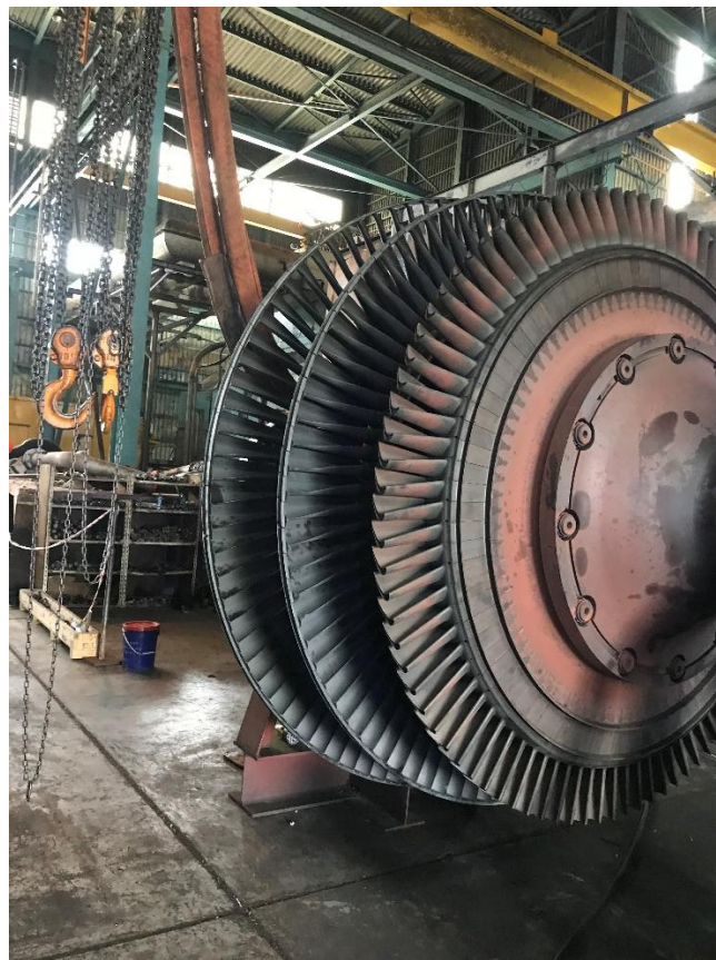
Figure 2.5 An image of the turbine section of a GE frame 9E gas turbine.
