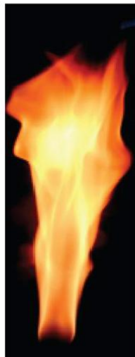
Figure 2.8 An image of a non-premixed flame. [43]
