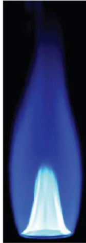
Figure 2.7 An image of a premixed flame. [43]
