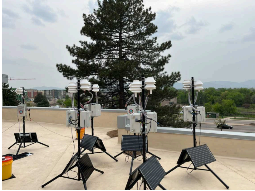
Figure S4 Image Illustrates the rooftop collocation effort done to check the capability of the sensors at the Powerhouse Campus, CSU, Colorado.
