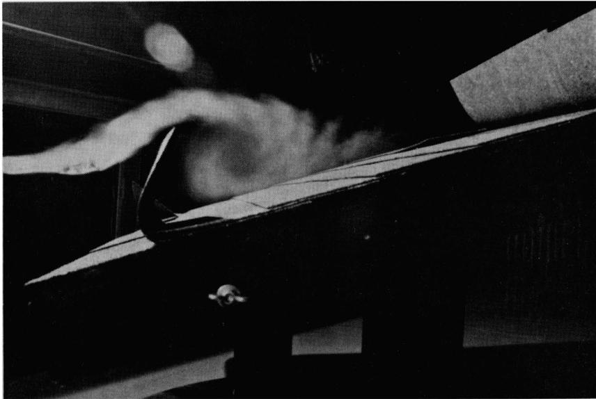
Figure 15a. Flow Visualization for 45° Yaw
