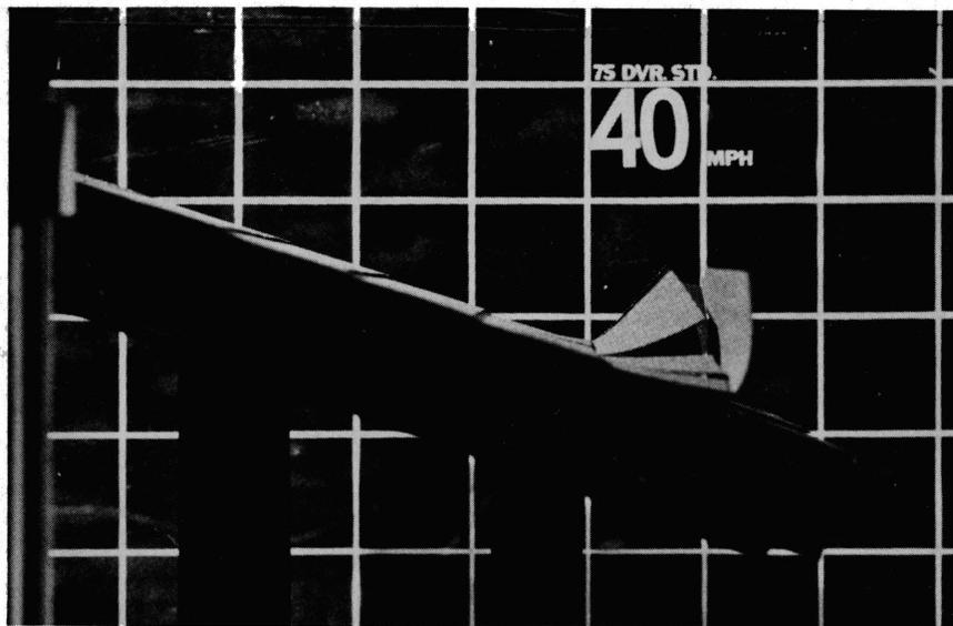
Figure 14a. Sequence of Shingle Lifting with Increasing Wind Speed
