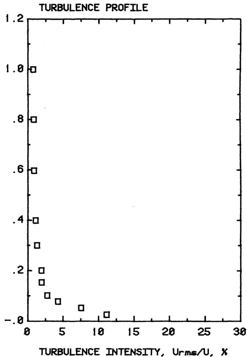
Figure 7. Mean Velocity and Turbulence Intensity Profiles near the Test Deck
