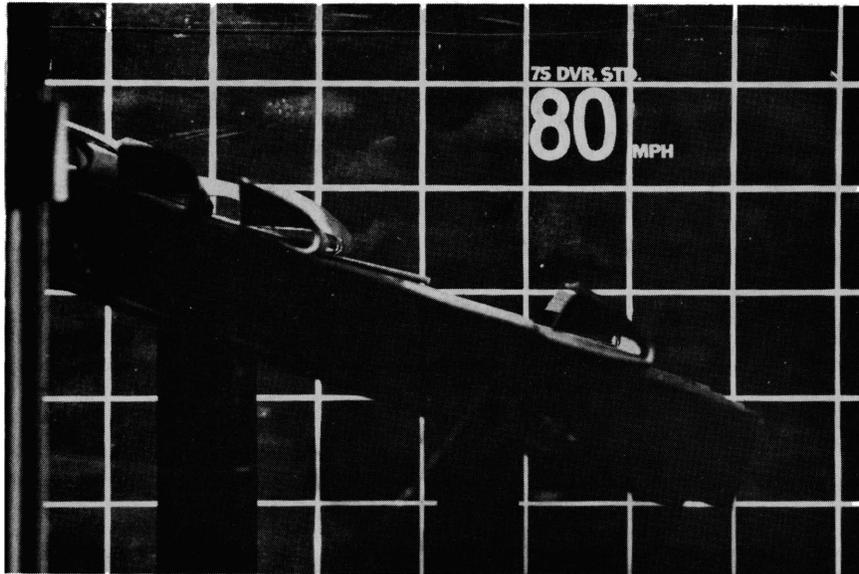
Figure 14c. Sequence of Shingle Lifting with Increasing Wind Speed
