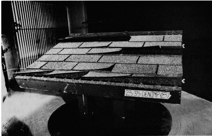
Figure 15b. Flow Visualization for 45° Yaw
