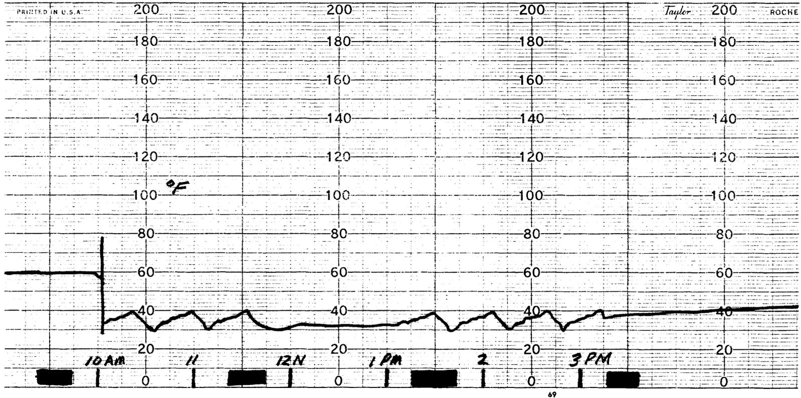
Figure 5a. Typical Temperature Record for Cold Test
