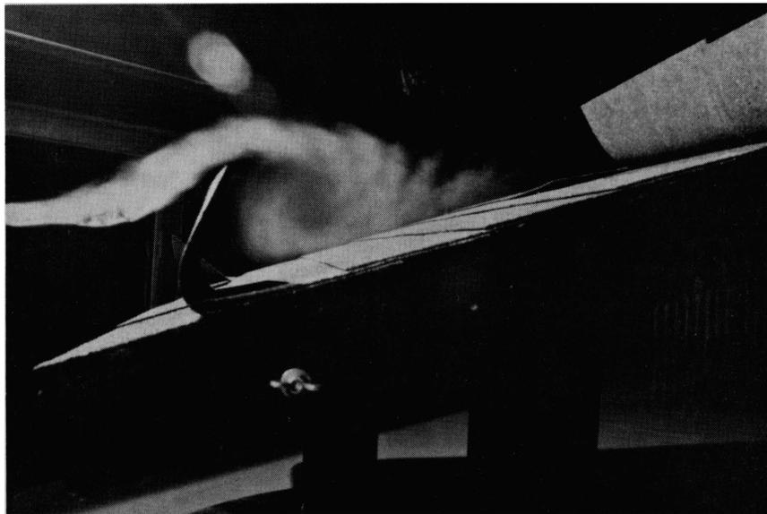
Figure 15a. Flow Visualization for 45° Yaw
