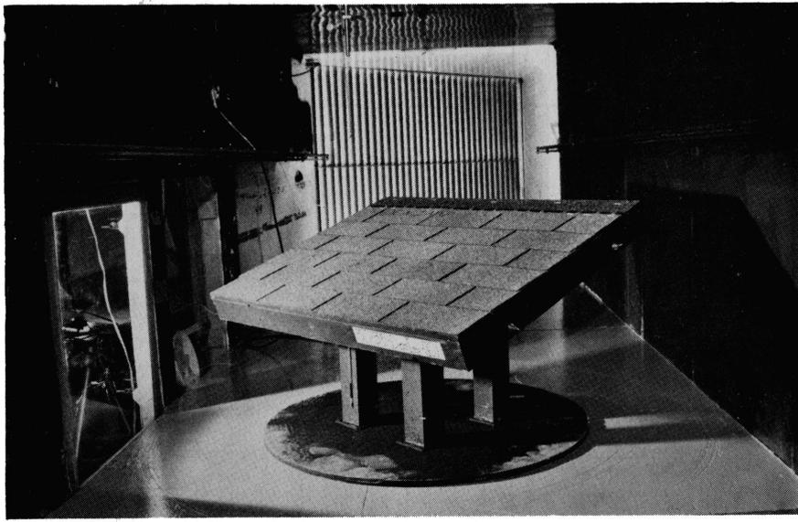
Test Stand with Shingle Deck at Yaw = 45 Degrees
