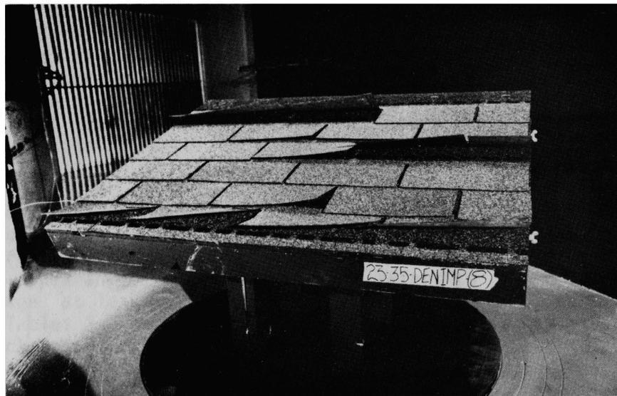
Figure 15b. Flow Visualization for 45° Yaw
