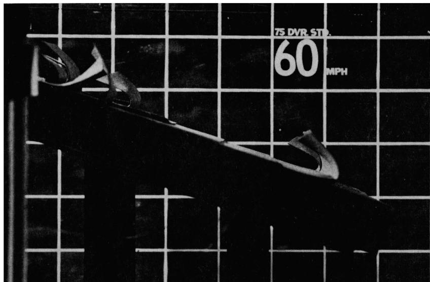
Figure 14b. Sequence of Shingle Lifting with Increasing Wind Speed
