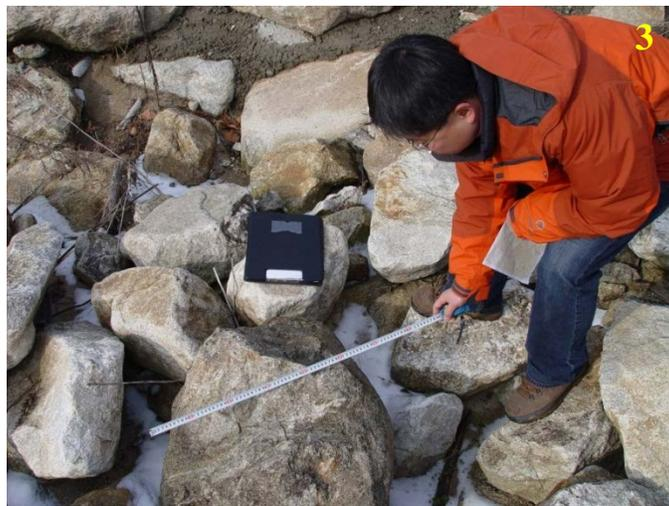
Figure 5.26. Bed material measurements in the Duksan Creek watershed
