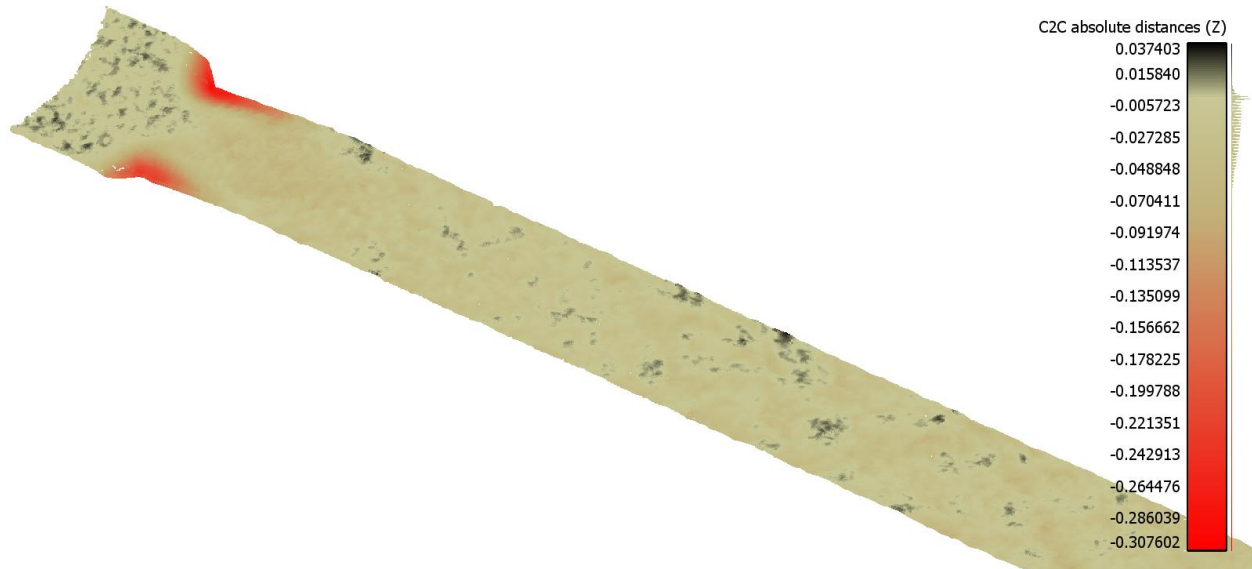
Figure D.47. Bed elevation difference between time zero and after 9-hour of experiments. (CW-0.75-2.72)
