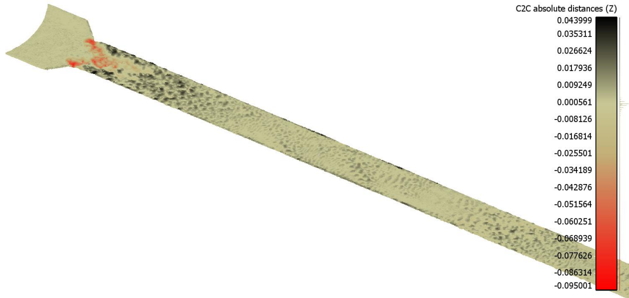
Figure D.9. Bed elevation difference between time zero and after 18-hour of experiments. (CW-0.50-0.30)
