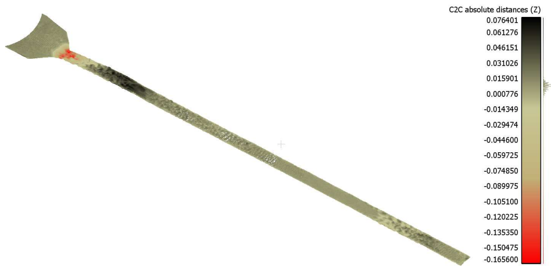
Figure D.28. LiDAR data at different time steps regarding long-contraction experiment; (a) 12th hour, (b) 24th hour, (c) 30th hour.
