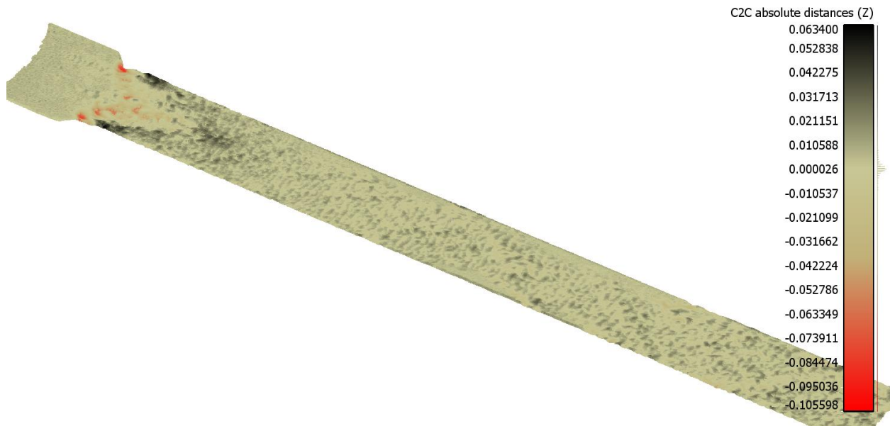
Figure D.21. Bed elevation difference between time zero and after 18-hour of experiments. (CW-0.75-0.72)
