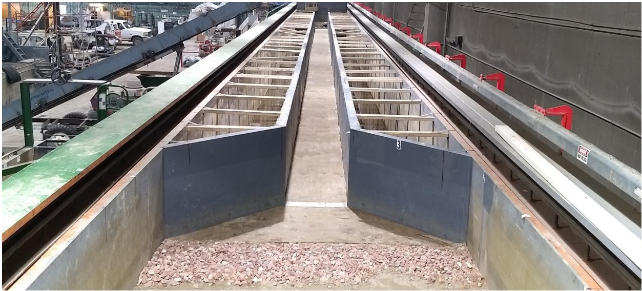
Figure 5.10. The contracted channel and its entrance covered with sheets of plywood that fixed the flat bed of the contracted section.
