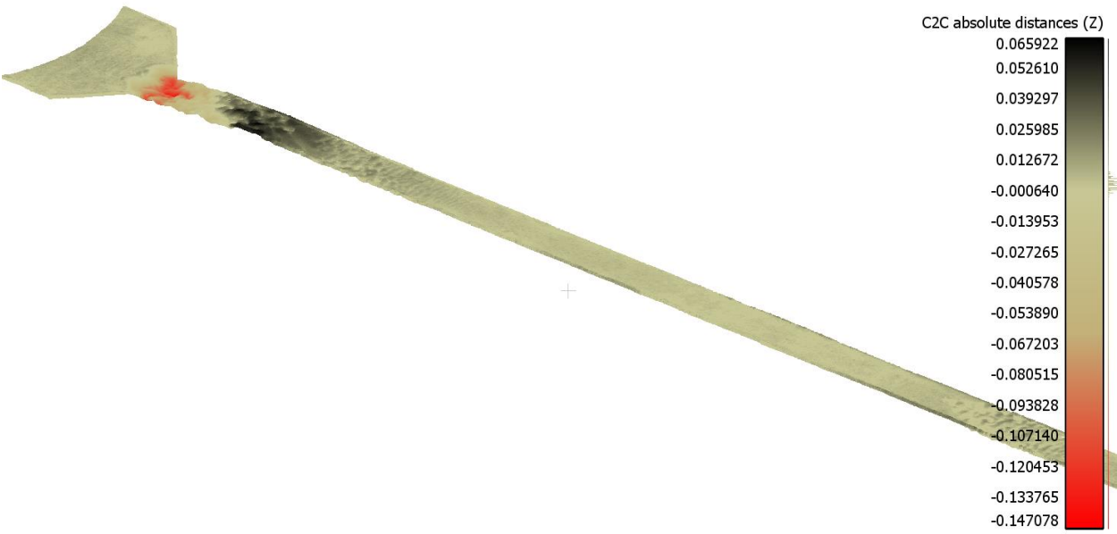
Figure D.27. Bed elevation difference between time zero and after 18-hour of long-contraction experiments. (CW-0.25-0.81)
