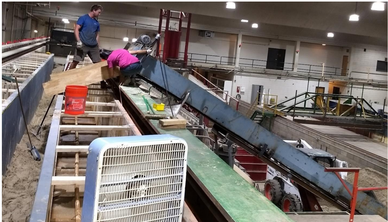
Figure 4.6. Conveying sand to the flume and placing the sand along the bed of the contracted channel; B_1/B_2 = 0.25 .
