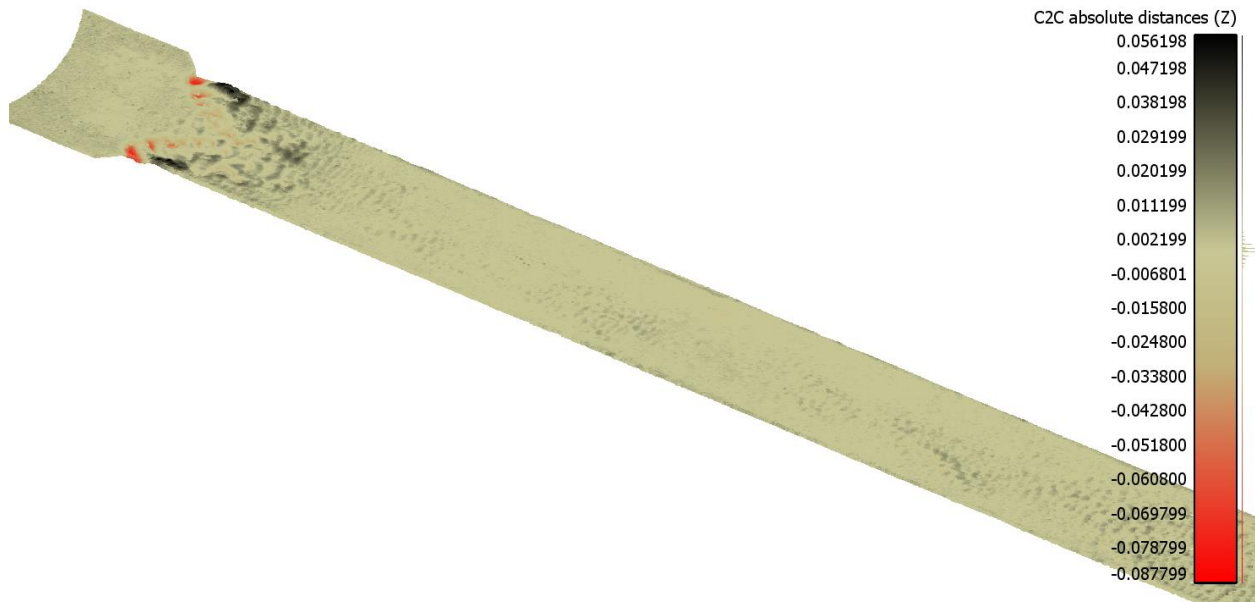
Figure D.18. Bed elevation difference between time zero and after 18-hour of experiments. (CW-0.75-0.56)
