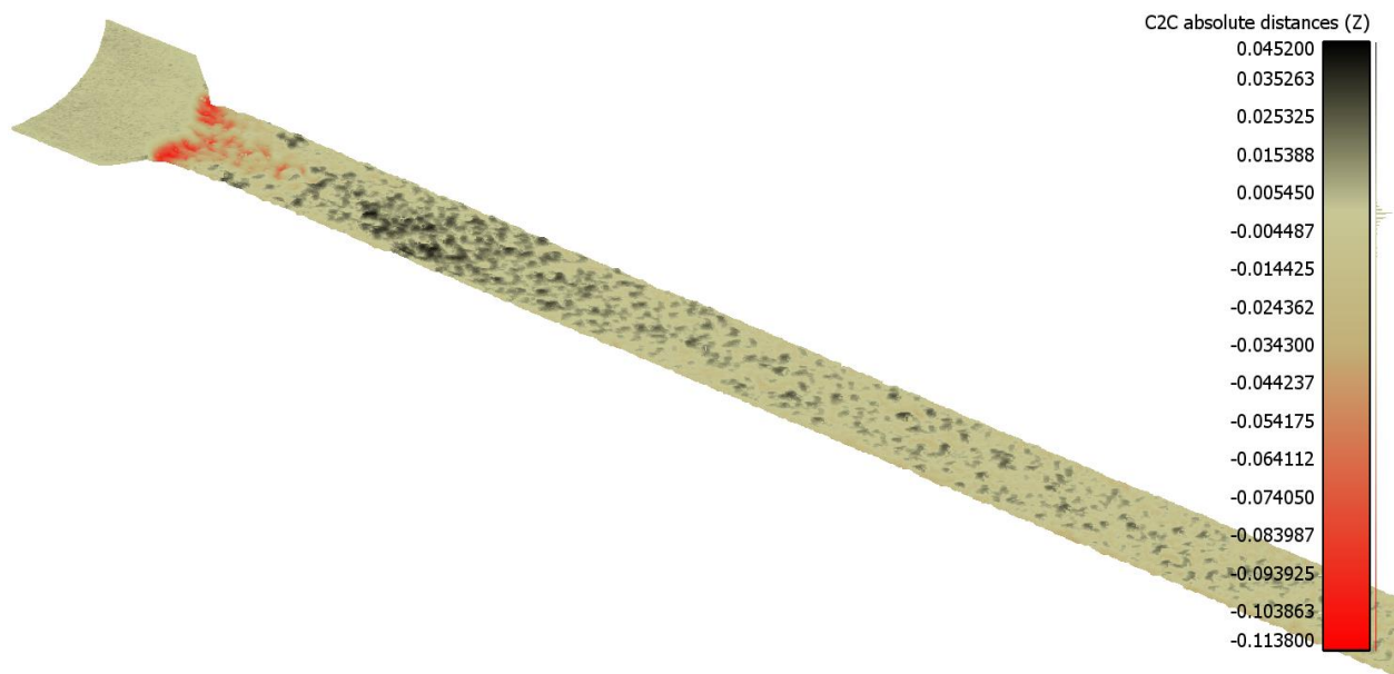
Figure D.12. Bed elevation difference between time zero and after 18-hour of experiments. (CW-0.50-0.42)
