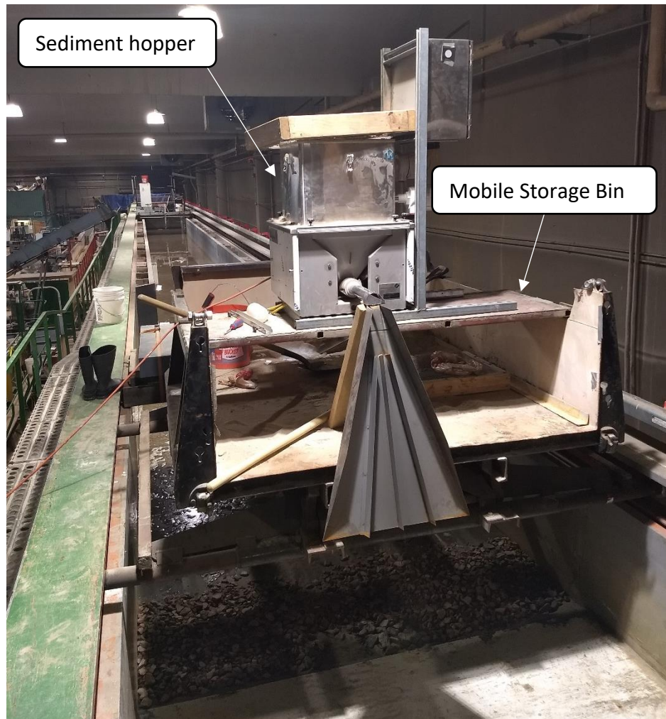
Figure 4.11. Positioning of the sediment hopper on the mobile, sediment-storage bin on the 2.44 m wide flume.
