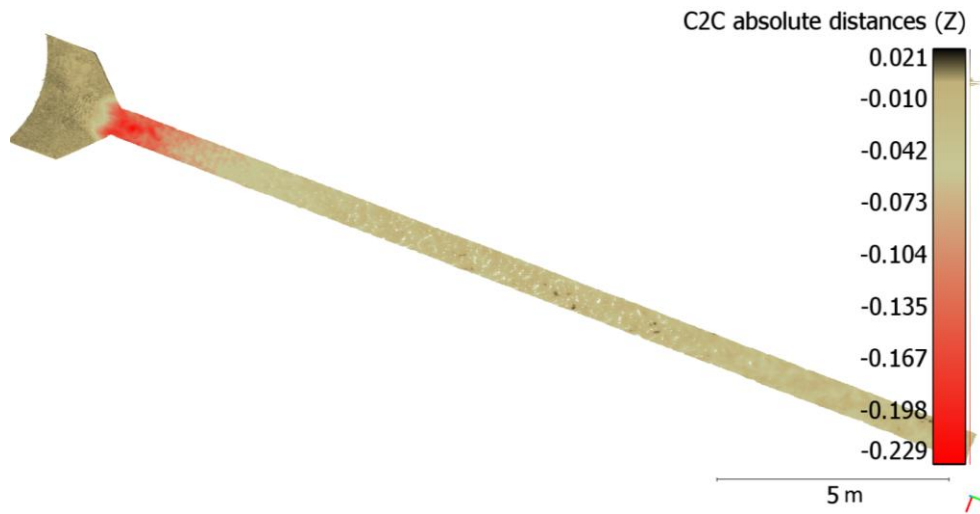
Figure 5.2. The LiDAR scan of the flume bed (CW- 0.25-0.30) after the 18 th hour of running. The red area indicates the region of deepest scour (The units of the scale are meters, and C2C means Cloud to Cloud, and is a term included in the LiDAR software used)
