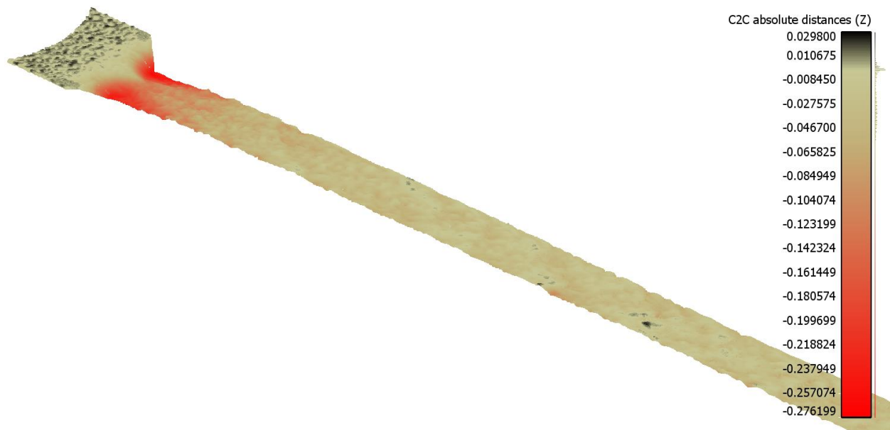
Figure D.29. Bed elevation difference between time zero and after 7-hour of experiments. (LB-0.50-1.44)
