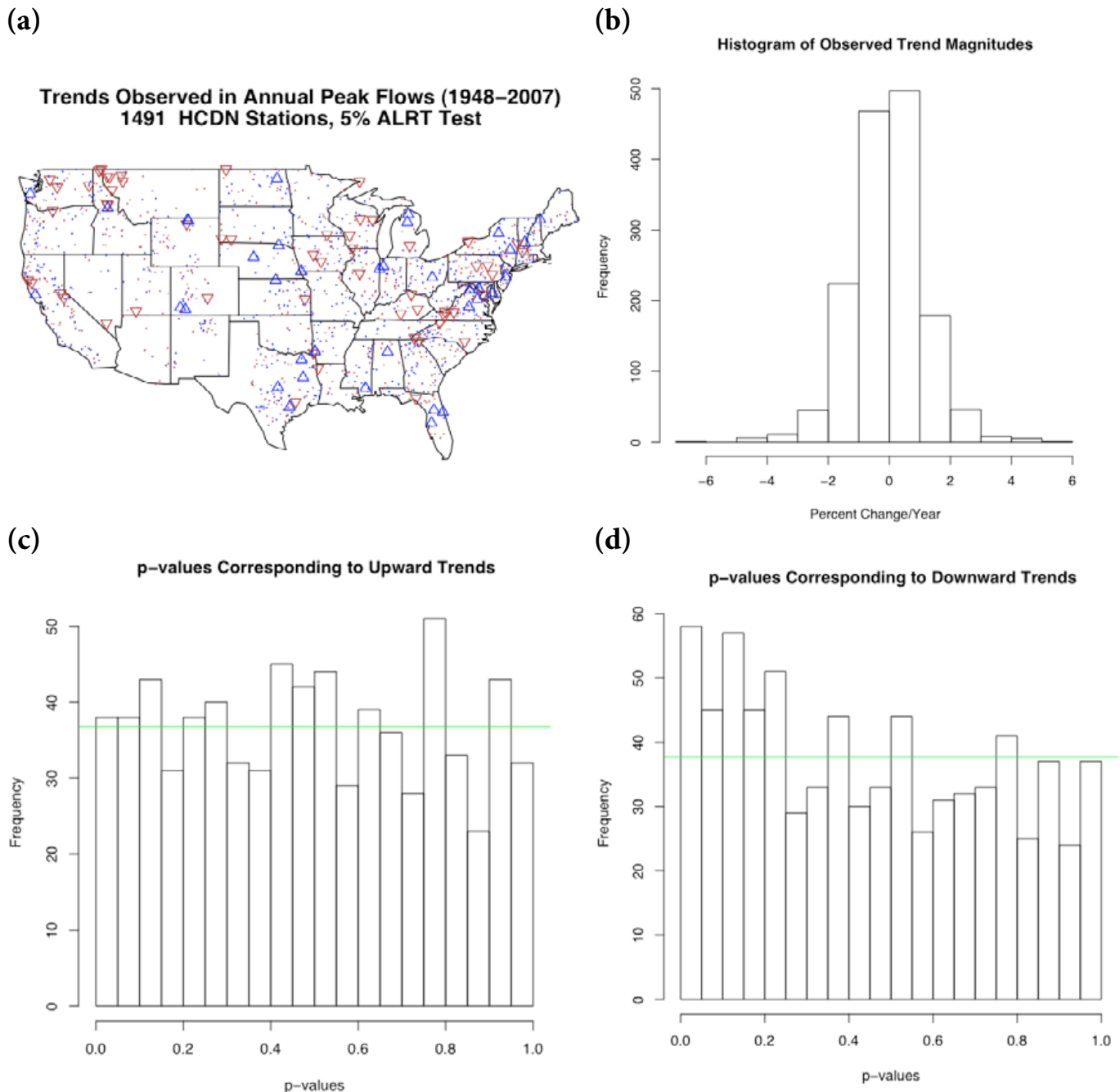
Figure 4. Summary of trends in annual instantaneous peak streamflow for the 60-year period 1948-2007 at 1491 stations from the USGS Hydro-Climatic Data Network (NCDN): a) trend direction and significance, with increasing trends in blue and decreasing trends in red, and those significant at the 0.05 level signified by open triangles (based on the Adjusted Likelihood Ratio Test [ALRT]); b) frequency distribution of trends by magnitude; c) frequency distribution of p-values associated with stations having increasing peak streamflow; and d) frequency distribution of p-values associated with stations having decreasing peak streamflow.
