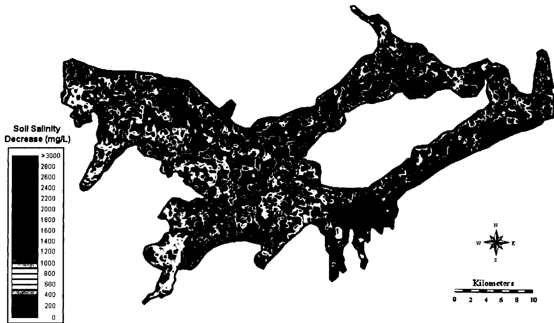
Figure L-39. 50% Recharge Reduction-90% Seepage Reduction-Subsurface Drainage Installation (50-m Spacing) Combination Scenario: Decrease in Soil Water Salinity over Irrigation Season 2001
