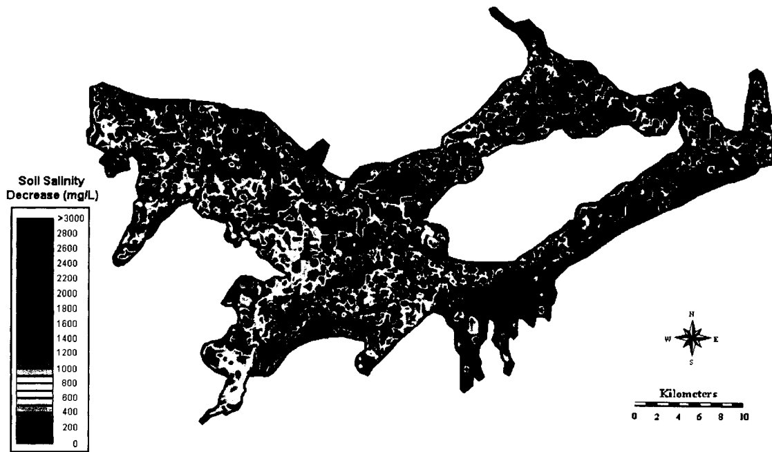
Figure L-45. 30% Recharge Reduction-50% Seepage Reduction-Subsurface Drainage Installation (100-m Spacing) Combination Scenario: Decrease in Soil Water Salinity over Irrigation Season 2001
