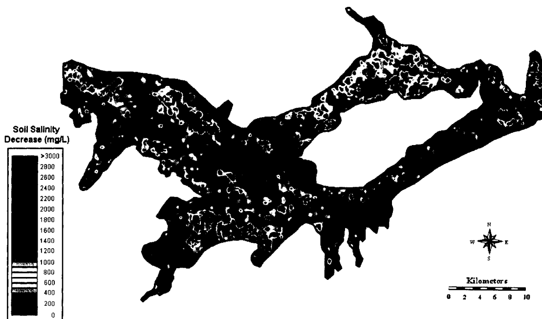
Figure L-37. 50% Recharge Reduction-90% Seepage Reduction-Subsurface Drainage Installation (50-m Spacing) Combination Scenario: Decrease in Soil Water Salinity over Irrigation Season 1999
