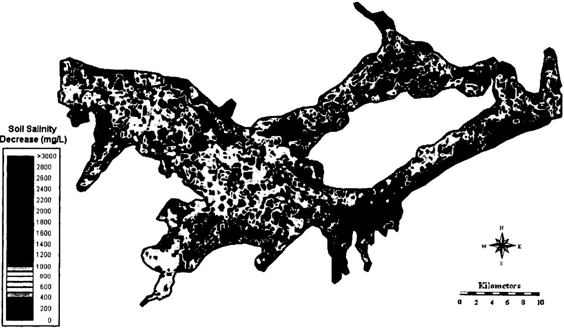
Figure L-44. 30% Recharge Reduction-50% Seepage Reduction-Subsurface Drainage Installation (100-m Spacing) Combination Scenario: Decrease in Soil Water Salinity over Irrigation Season 2000
