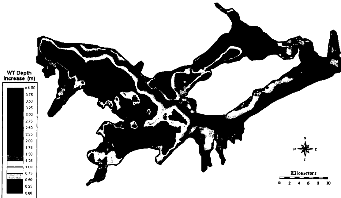
Figure L-36. 50% Recharge Reduction-90% Seepage Reduction-Subsurface Drainage Installation (50-m Spacing) Combination Scenario: Increase in Water Table Depth over Irrigation Season 2001
