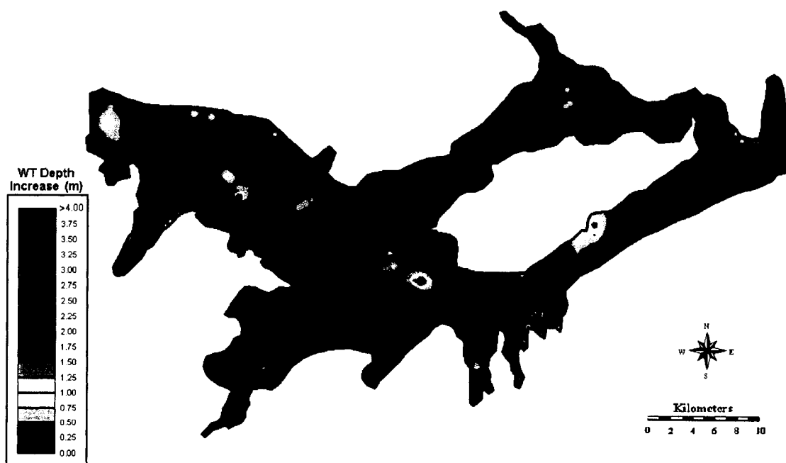
Figure L-28. 200% Pumping Volume Increase Scenario: Increase in Water Table Depth over Irrigation Season 1999
