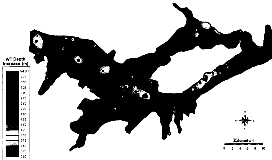
Figure L-29. 200% Pumping Volume Increase Scenario: Increase in Water Table Depth over Irrigation Season 2000
