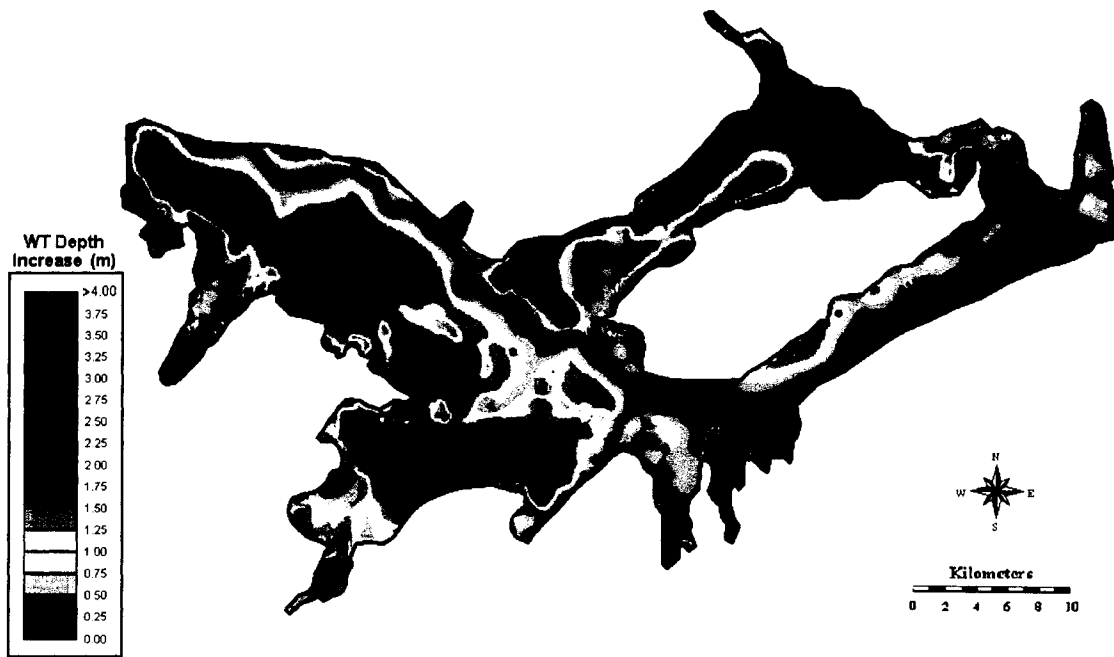
Figure L-35. 50% Recharge Reduction-90% Seepage Reduction-Subsurface Drainage Installation (50-m Spacing) Combination Scenario: Increase in Water Table Depth over Irrigation Season 2000
