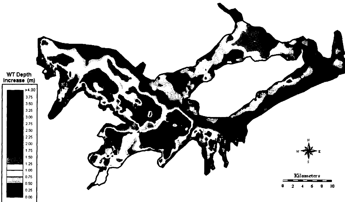
Figure L-42. 30% Recharge Reduction-50% Seepage Reduction-Subsurface Drainage Installation (100-m Spacing) Combination Scenario: Increase in Water Table Depth over Irrigation Season 2001
