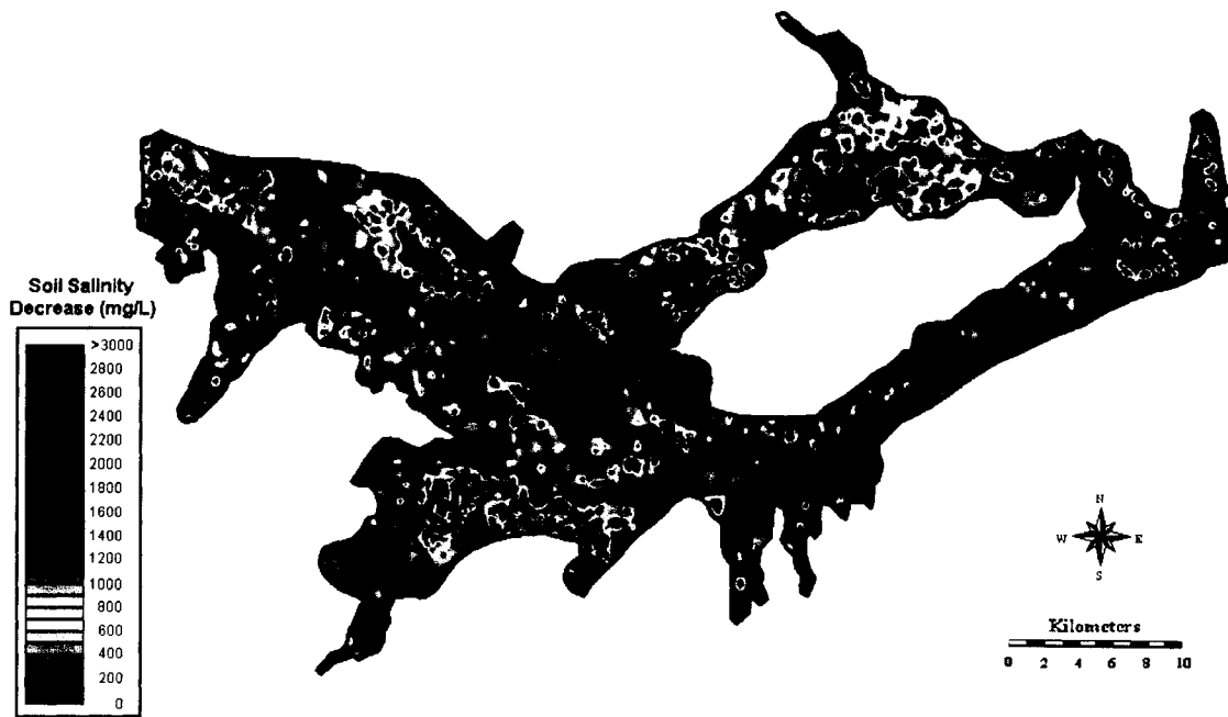
Figure L-49. 50% Recharge Reduction-90% Seepage Reduction Combination Scenario: Decrease in Soil Water Salinity over Irrigation Season 1999
