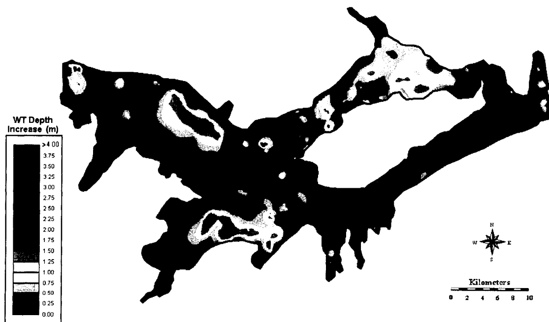
Figure L-22. Subsurface Drainage (50-m Spacing) Scenario: Increase in Water Table Depth over Irrigation Season 1999
