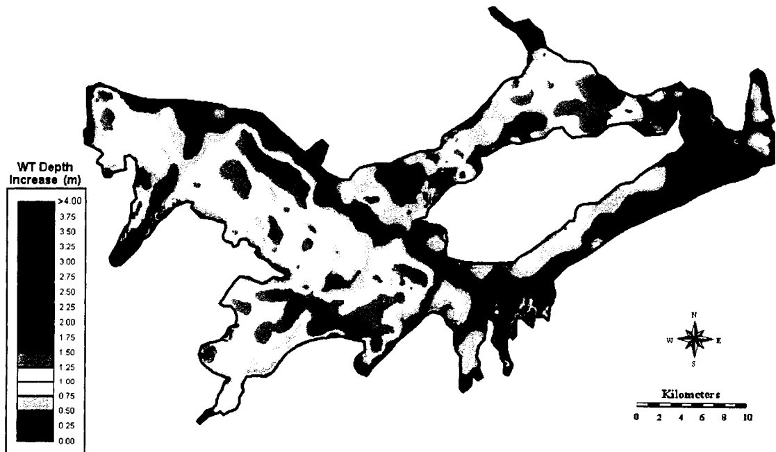
Figure L-40. 30% Recharge Reduction-50% Seepage Reduction-Subsurface Drainage Installation (100-m Spacing) Combination Scenario: Increase in Water Table Depth over Irrigation Season 1999
