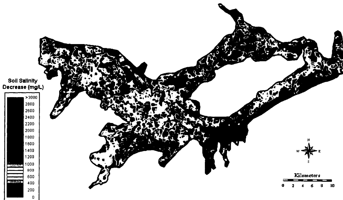
Figure L-38. 50% Recharge Reduction-90% Seepage Reduction-Subsurface Drainage Installation (50-m Spacing) Combination Scenario: Decrease in Soil Water Salinity over Irrigation Season 2000
