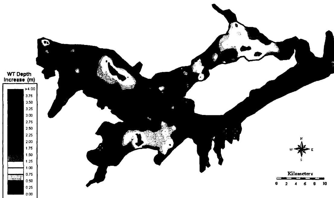
Figure L-23. Subsurface Drainage (50-m Spacing) Scenario: Increase in Water Table Depth over Irrigation Season 2000
