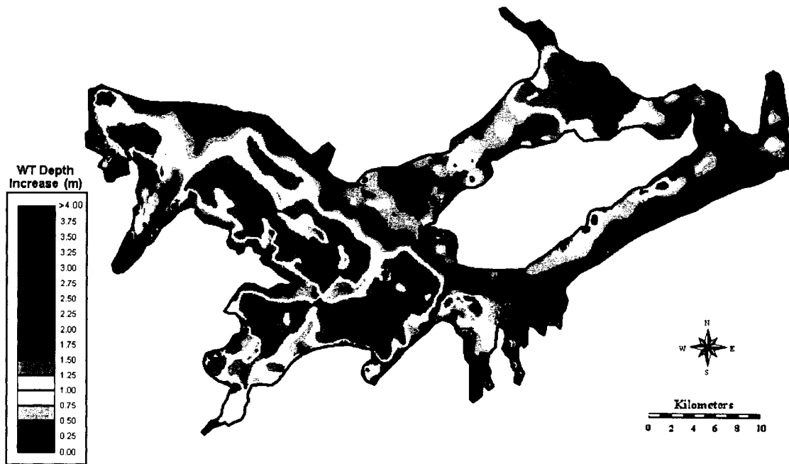
Figure L-41. 30% Recharge Reduction-50% Seepage Reduction-Subsurface Drainage Installation (100-m Spacing) Combination Scenario: Increase in Water Table Depth over Irrigation Season 2000
