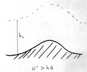
where  $\Delta = g\Delta\rho/\rho$ . If we define a Richardson number as  $Ri_0 = h\Delta/u^2$ , there exists a critical value of  $Ri_0 = 1$ , where the flow will not go over the hill. Simple minded theories won't get the flow over hills greater than about 200 meters.
