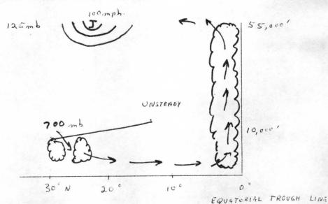
A schematic diagram of the zonally averaged equatorial zone is shown above. There is no heat flow across the equatorial trough line, although there is across the geographical equator. The rising portions of the Hadley cell are confined to restricted regions of active "hot towers" in which undilute sub-cloud air is pumped to great heights. Only 1500 to 5000 "hot towers" need to exist, on an average, in order to complete the energy balance requirements.
