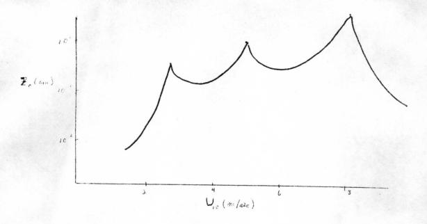
The peaks in  $z_0$  indicate the possible existence of critical wind speeds. A list of references is included at the end of this report.
