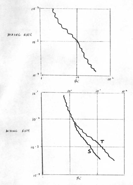
The curve denoted by T corresponds to interfaces associated with a temperature difference, while the curve denoted by s is associated with a salinity difference. These results indicate that heat diffuses faster than salt. If  $\mathbf{u}_{\mathbf{g}}$  represents the velocity of the grid,
