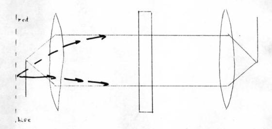
The ordinary Schlieren knife edge is replaced by a filter with red on top, blue on the bottom, and yellow on one side. Changes in density affect the path of light rays. Blue corresponds to a stable gradient and red an unstable density gradient. Horizontal density gradients will be indicated by the yellow coloring.
