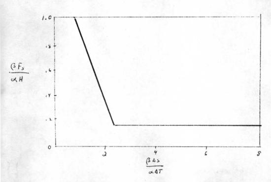
For a fluid of given properties and in the high Rayleigh number limit, the flux will depend upon  $\Delta T$  and  $\Delta s$ . However the rate at which the flux dilutes will depend on the depth. Properties will change more rapidly in a shallow layer than in a deep layer.
