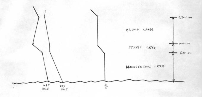
A mean schematic diagram of the trade wind boundary layer is shown above, where the boundary layer is defined as the layer in which the winds depart from their geostrophic values.
