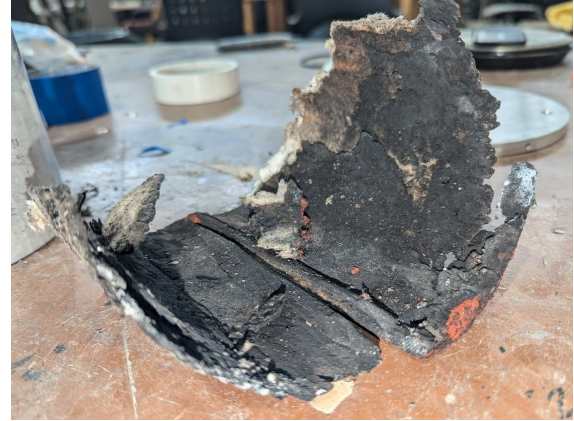
Figure 4.27: Combustion chamber liner condition after test fire
