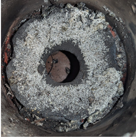
Figure 4.28: Liner material collected and melted on the converging section of the nozzle
