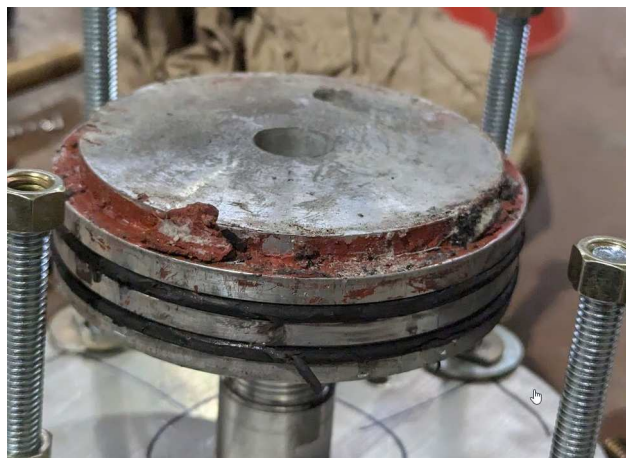
Figure 4.25: O-ring damage seen on the injector plate
