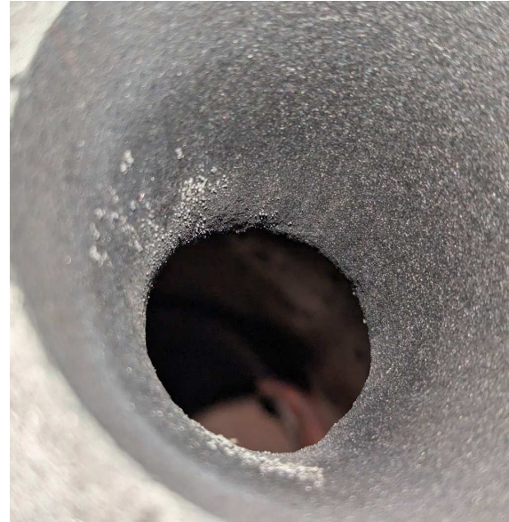
Figure 4.29: Throat ablation seen in the sharp edge and the non-circularity
