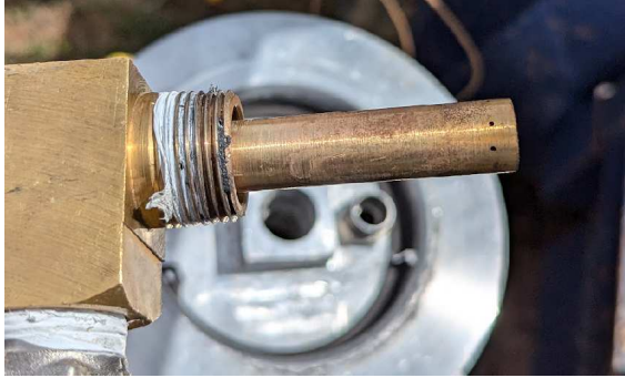
Figure 4.15: Soot found on the surface of the pintle injector
