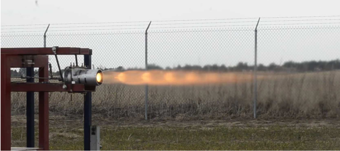
Figure 4.17: Static fire of the ACMPE on the second static fire test
