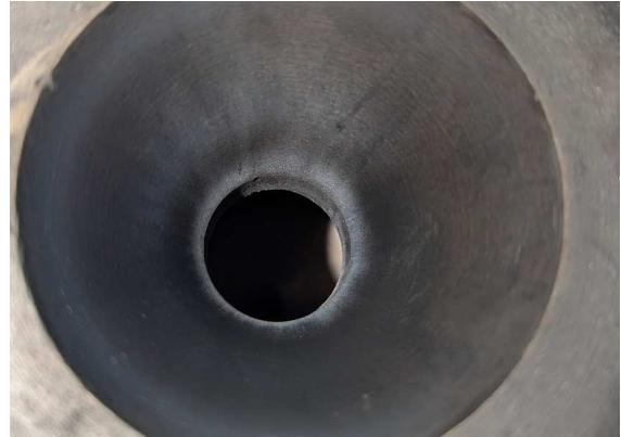
Figure 4.16: Graphite nozzle condition after first static fire test
