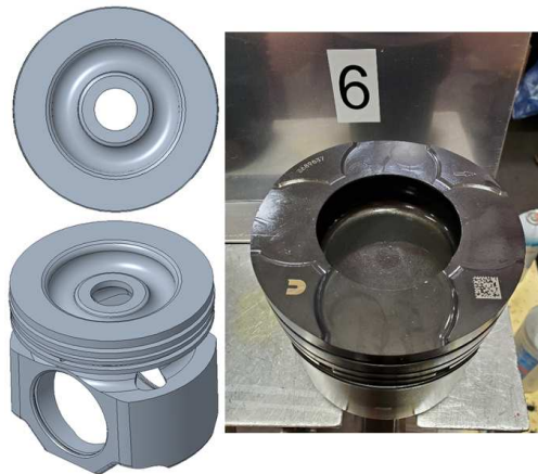
Figure 3.4: Pistons used in deactivated cylinders 1-5 (left). Baseline SI-NG piston design used in firing cylinder 6 (right).
