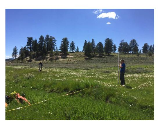
Figure 3: Surveying the channel cross-section. Flow is right to left.
