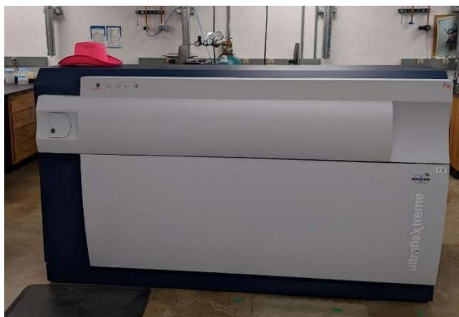
Figure 78: Bruker UltraFlextreme MALDI-TOF-MS. Located in the ARC. Image acquired by Ph.D. Candidate Mueller.
