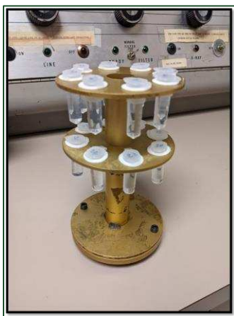
Figure 16: Sample carousel with top and bottom rows holding additively manufactured sample holders (white) and microcentrifuge tubes containing Fricke solution.
