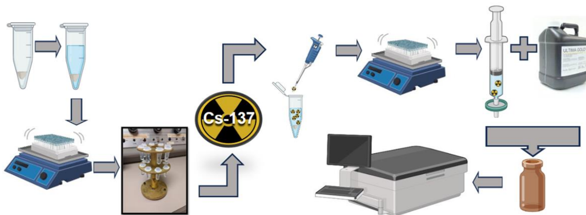
Figure 25: Pictorial representation of batch-contact studies used for contacting plutonium-239 with EXC resins post-irradiation.
