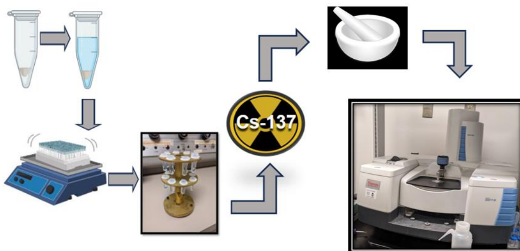
Figure 65: Pictorial representation of batch studies with the irradiation of EXC resins and FTIR analysis.
