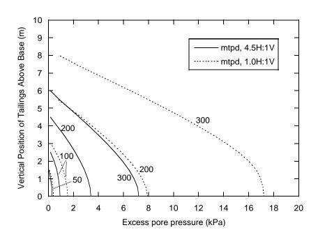
**Fig. 4.9.** Profiles of excess pore pressure at an elapsed time of 1.4 yr (500 d) based on model simulations in FSConsol for gradual tailings deposition into an inverted square frustum with a 100-m-wide base, 10-m-tall sides slopes, and horizontal (H) to vertical (V) sideslope configurations of 1.0H:1.0V and 4.5H:1.0V. Results presented for tailings production rates ranging from 50 to 300 mtpd.
