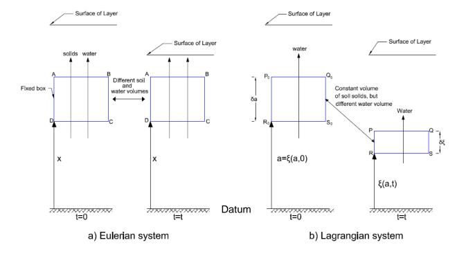
**Fig. 2.1.** Schematics of Eulerian and Lagrangian coordinate systems from Schiffman et al. (1988). Definitions: x = Eulerian coordinate, distance of fixed element from datum plane, a = initial state Lagrangian coordinate,  $\xi (a,t) = \text{convective}$  coordinate as function of a and time t,  $\delta a = \text{thickness}$  of  $P_0Q_0R_0S_0$  element, and  $\delta \xi = \text{thickness}$  of PQRS element.
