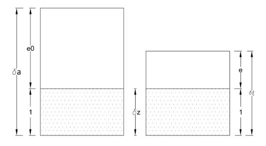
Fig. 2.2. Schematic of coordinate relationships and void ratio change during consolidation from Schiffman et al. (1988). Definitions: z = solids coordinate,  $e_o = initial$  void ratio , and  $\xi = convective$  coordinate.
