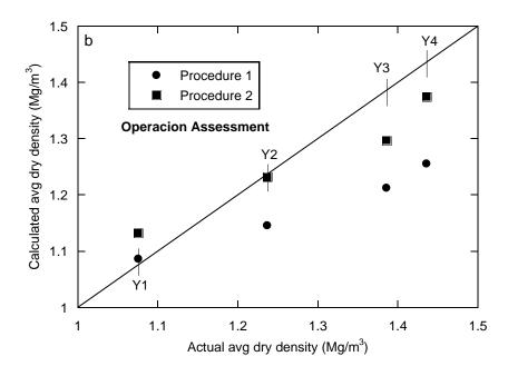
**Fig. 4.12.** Comparison of predicted average dry tailings density to actual tailings dry density in the full-scale tailings storage facility. Model simulation results representative of the first four years shown for the (a) Design assessment and (b) Operation assessment with a cyclone operation time (COT) of 70 % considering dry density calculation Procedures 1 and 2 (Fig. 3.13). Yi = Year i (i=1, 2, 3, 4)
