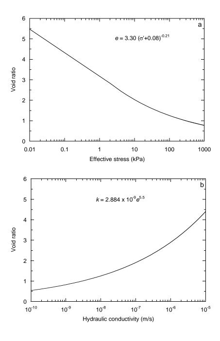
**Fig. 3.5.** Constitutive relationships from Gjerapic et al. (2008) used in the gradual tailings deposition benchmark example: (a) effective stress versus void ratio and (b) hydraulic conductivity versus void ratio.
