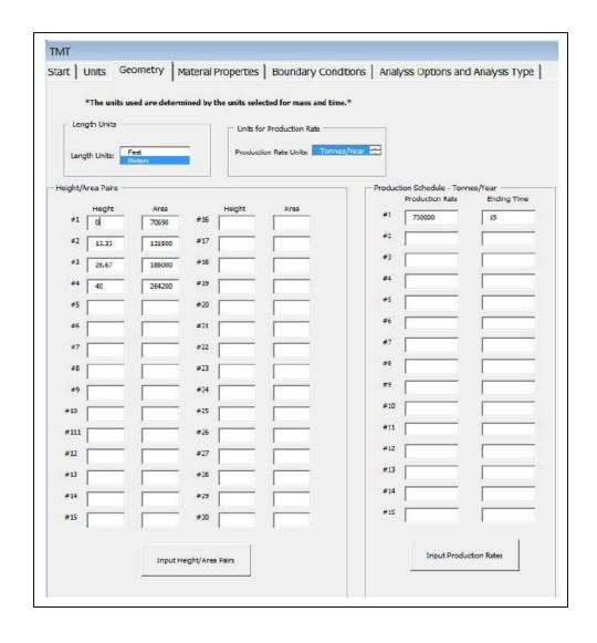
**Fig. A.2.** TMT geometry tab where height-area pairs and production schedule can be entered (figure from Miller 2012).
