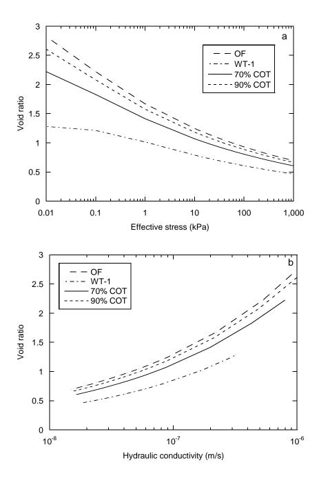
**Fig. 3.11.** Constitutive relationships for impounded tailings used in the Design Assessment with 70 and 90 % cyclone operation time (COT) assumed during the entire operation life of the facility: (a) effective stress versus void ratio and (b) hydraulic conductivity versus void ratio. Relationships computed by using a weighted average of OF and WT-1 are labeled as 70% COT and 90% COT curves.
