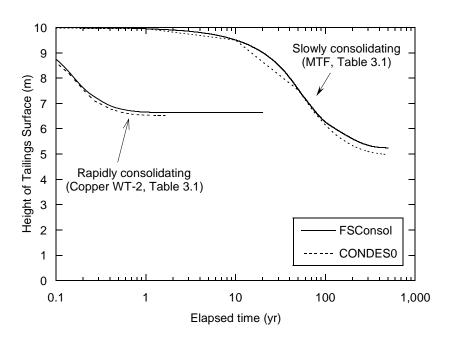
**Fig. 4.3.** Temporal trends of tailings surface height (i.e., settlement) for model simulations conducted in CONDESO and FSConsol for an instantaneously filled column considering slowly consolidating tailings (SCT) with  $k = 1.10 \times 10^{-11} \cdot e^{3.79}$  (m/s) and rapidly consolidating tailings (RCT) with  $k = 1.02 \times 10^{-7} \cdot e^{3.42}$  (m/s). Note:  $k = 1.02 \times 10^{-11} \cdot e^{3.42}$  (m/s) and conductivity and  $e = 1.02 \times 10^{-11} \cdot e^{3.42}$  (m/s).
