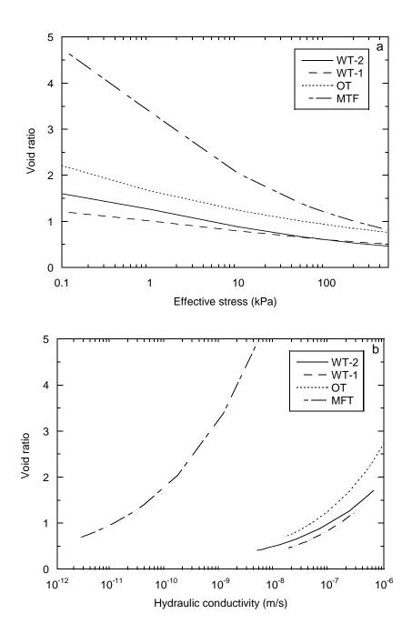
**Fig. 3.1.** Constitutive relationships for mine tailings used in the parametric study and case study: (a) effective stress versus void ratio relationships and (b) void ratio versus hydraulic conductivity relationship. Note: WT-1 = copper whole tailings from pilot-scale evaluation, WT-2 = copper whole tailings from full-scale operation, OT = copper overflow tailings, and MFT = oil sand mature fine tailings.
