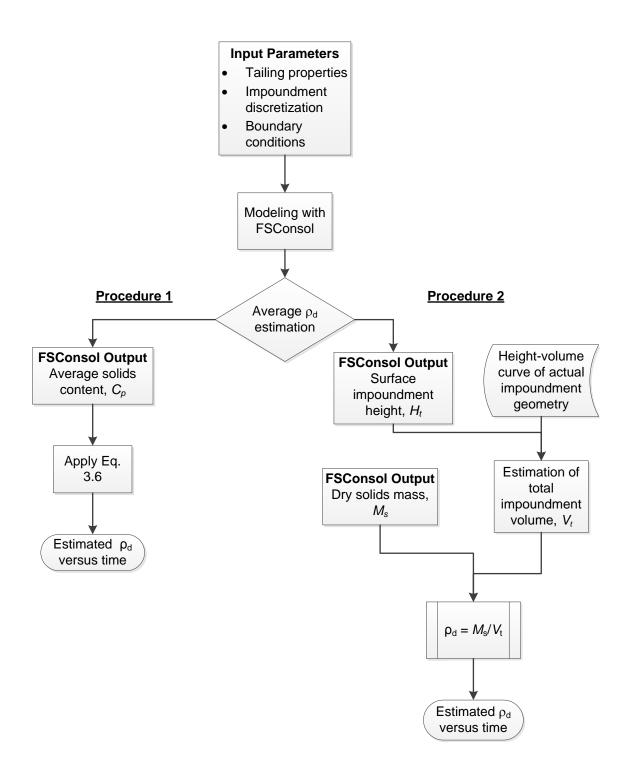
**Fig. 3.13.** Flow chart of dry density estimation techniques, Procedure1 and Procedure 2, based on FSConsol output and actual height-volume relationship of the full-scale tailings storage facility.
