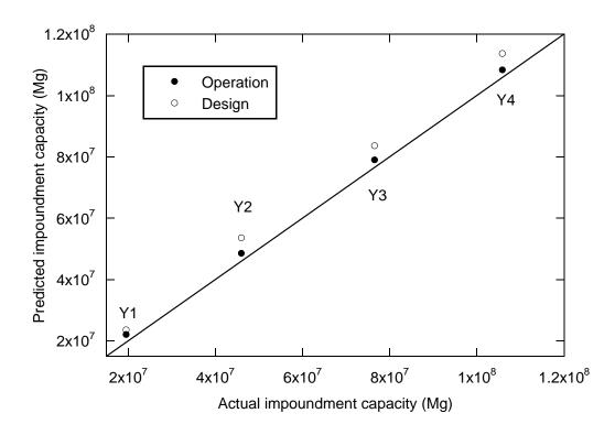
**Fig. 4.13.** Comparison of predicted impoundment capacity to actual impoundment capacity of the full-scale tailings storage facility. Model simulation results representative of the first four years shown for the (a) Design assessment and (b) Operation assessment with a cyclone operation time (COT) of 70 %. Yi = Year i (i=1, 2, 3, 4)
