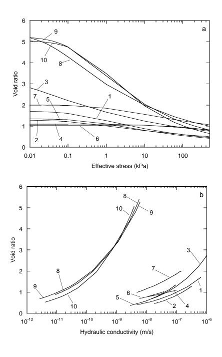
**Fig. A.1.** Compilation of constitutive relationships of mine tailings (Table A.1) (a) effective stress - void ratio relationship (b) hydraulic conductivity – void ratio relationship.
