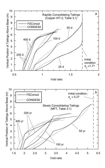
**Fig. 4.5.** Profiles of void ratio at different elapsed times based on model simulations in CONDES0 and FSConsol of an instantaneously filled column considering (a) rapidly consolidating tailings ( $e = 1.30 \ (\sigma' + 0.192)^{-0.168}$ ) and (b) slowly consolidating tailings ( $e = 3.52 \ (\sigma' + 0.181)^{-0.236}$ ).
