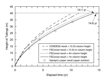
**Fig. 4.2.** Temporal relationships of tailings height for the continuous tailings deposition benchmark example in Gjerapic et al. (2008). Model simulations shown for FSConsol considering impoundment discretized into 1-m-, 4-m-, and 13.33-m-tall columns; CONDESO results only based on impoundment discretization into three 13.33-m-tall columns. Continuous deposition was stopped once height of tailings = 40 m; thus, stop time in simulation = filling time.
