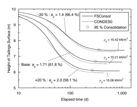
**Fig. 4.6.** Temporal trends of tailings surface height based on model simulations in FSConsol and CONDESO of an instantaneously filled column considering different initial void ratio (*e<sub>o</sub>*) for copper whole tailings (WT-2). Circle on curve represents time at which 95% consolidation is achieved; average dry densities (*p<sub>d</sub>*) listed for complete consolidation.
