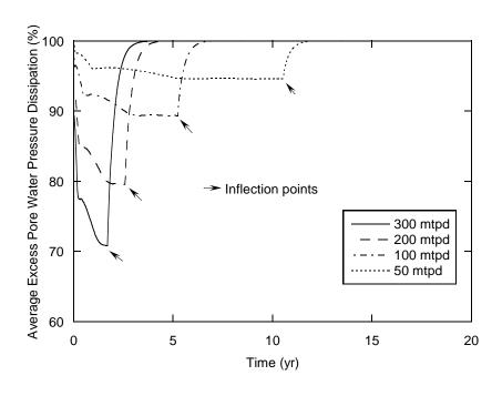
**Fig. 4.10.** Temporal relationships of average excess pore water pressure dissipation based on model simulations in FSConsol for gradual tailings deposition into an inverted square frustum with a 100-m-wide base, 10-m-tall sides slopes, and horizontal (H) to vertical (V) side-slope configuration of 1.0H:1.0V. Results presented for tailings production rates ranging from 50 to 300 mtpd and the inflection point represents time to reach complete filling of the impoundment.
