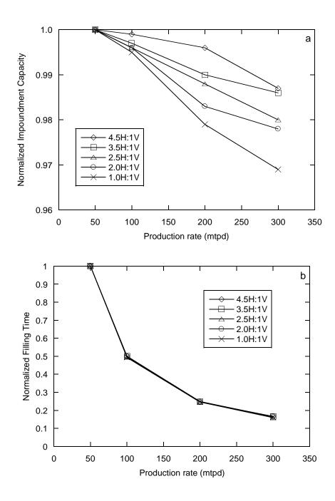
**Fig. 4.8.** Relationships of normalized impoundment capacity and normalized filling time as a function of tailings production rate based on model simulations in FSConsol for graduate tailings deposition into an inverted square frustum with a 100-m-wide base, 10-m-tall sides slopes, and different horizontal (H) to vertical (V) side-slope configurations. Capacity and filling time normalized to results for a tailings production rate of 50 mtpd.
