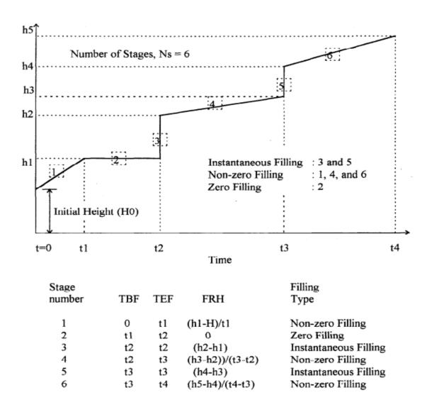
**Fig. 3.3.** Deposition chart of nominal height versus time and input table for staged filling used in CONDES0 (Yao and Znidarcic 1997).
