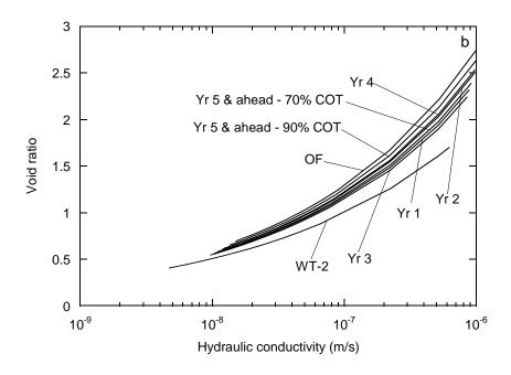
**Fig. 3.12.** Constitutive relationships for impounded tailings used in the Operation Assessment with 70 and 90 % COT assumed for Year 5 to the end of operation: (a) effective stress versus void ratio and (b) hydraulic conductivity - void ratio. All curves, with exception of OF and WT-2, were used in the models and developed from a weighted average of OF and WT-2.
