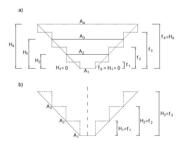
**Fig. 3.2.** Geometrical discretization schemes of (a) a tailings impoundment assuming four filling stages (upper bound solution in Gjerapic et al. 2008) and (b) general configuration assumed in FSConsol (figures from Coffin 2010): Note:  $H_{i}$  = column height,  $f_{i}$  = interstage heights at which the filling rate changes, and  $A_{i}$  = deposition area for each column.
