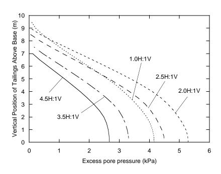
**Fig. 4.7.** Profiles of excess pore pressure at an elapsed time of 5.5 yr (2000 d) based on model simulations in FSConsol for gradual tailings deposition into an inverted square frustum with a 100-m-wide base, 10-m-tall sides slopes, and different horizontal (H) to vertical (V) side-slope configurations.
