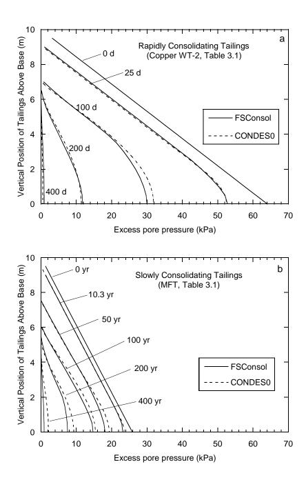
**Fig. 4.4.** Profiles of excess pore water pressure  $(u_e)$  at different elapsed times based on model simulations in CONDESO and FSConsol of an instantaneously filled column considering (a) rapidly consolidating tailings (RCT) and (b) slowly consolidating tailings (SCT).
