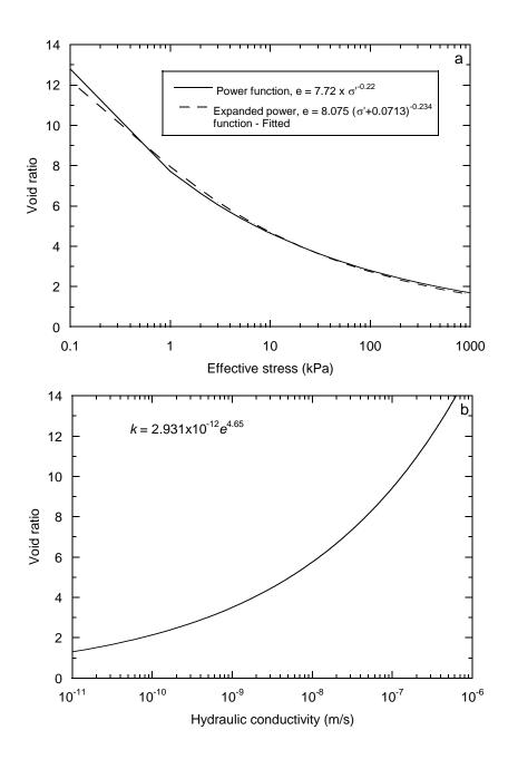
**Fig. 3.4.** Constitutive relationships from Townsend and McVay (1990) used in the instantaneous tailings deposition benchmark example: (a) effective stress versus void ratio relationship with power function based on Eq. 2.7 and expanded power function based on Eq. 2.8, and (b) hydraulic conductivity versus void ratio relationship with power function relationship based on Eq. 2.9.
