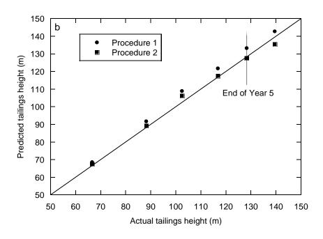
**Fig. 4.15.** Comparison of predicted tailings height to actual tailings height of the full-scale tailings storage facility. Model simulation results representative of the first six years shown for the (a) Design assessment and (b) Operation assessment with a cyclone operation time (COT) of 70 % and Procedure 1 and 2.
