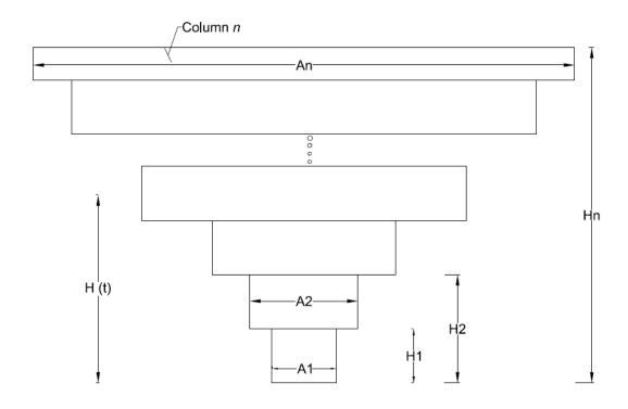
**Fig. 3.10.** Geometrical discretization of the full-scale copper tailings impoundment for the numerical simulations. Notes:  $H_{(t)}$  tailings surface height at time t;  $H_i$ ,  $A_i$  are column height and surface area of column i, respectively.
