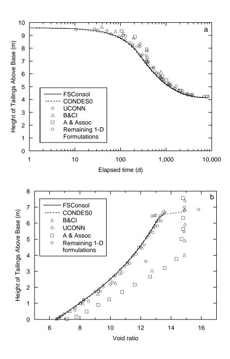
**Fig. 4.1.** One-dimensional consolidation modeling results for the instantaneous benchmark example in Townsend and McVay (1990): (a) temporal trends of height of tailings from twelve predictions in Townsend and McVay (1990), CONDESO, and FSconsol; and (b) void ratio profiles the end of Year 1 for ten predictions in Townsend and McVay (1990), CONDESO, and FSConsol.
