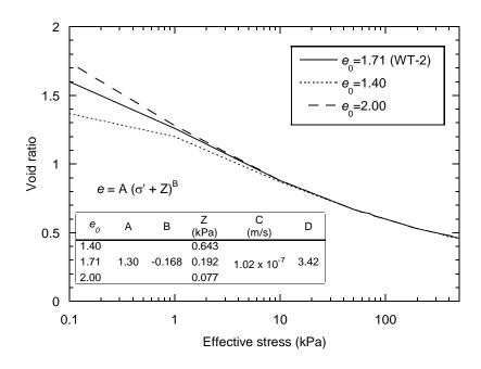
**Fig. 3.6.** Effective stress versus void ratio relationships of copper tailings (WT-2, Table 3.1) for initial void ratios (e₀) of 1.4 (- 20 %), 1.71 (base case), and 2.0 (+ 20 %).
