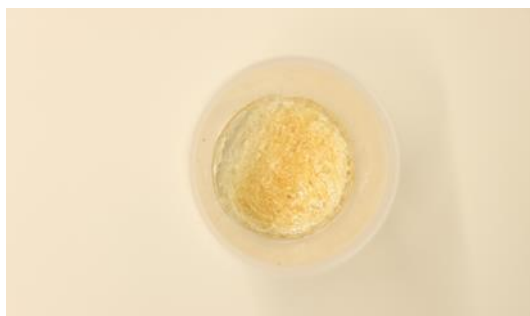
Figure 6.8. a) TMPTA monomer containing 0.2 phr BPO and DMA/BPO of 4 mol/mol spontaneously polymerized upon addition of redox initiator.
