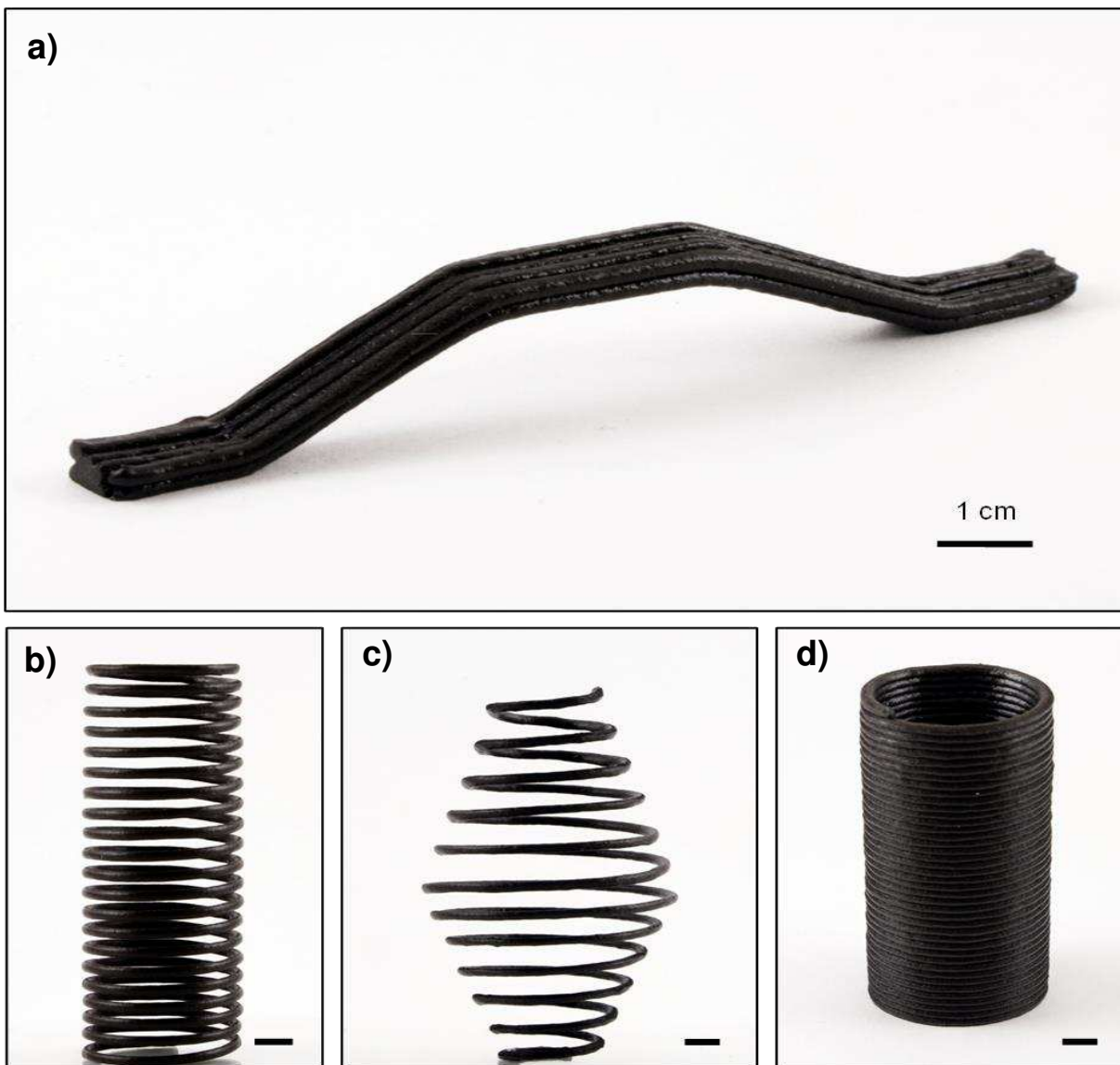
Figure 5.2. Additive manufacturing of complex geometries using the developed laser assisted printing technique with the ink containing 15 vol% CF. (a) An example of a multi-layer object printed linearly in the air. (b, c, d) Samples were printed on a rotating platform while the nozzle moved in the x-z plane at varying speeds. Scale bar in b–c represents 5 cm.
