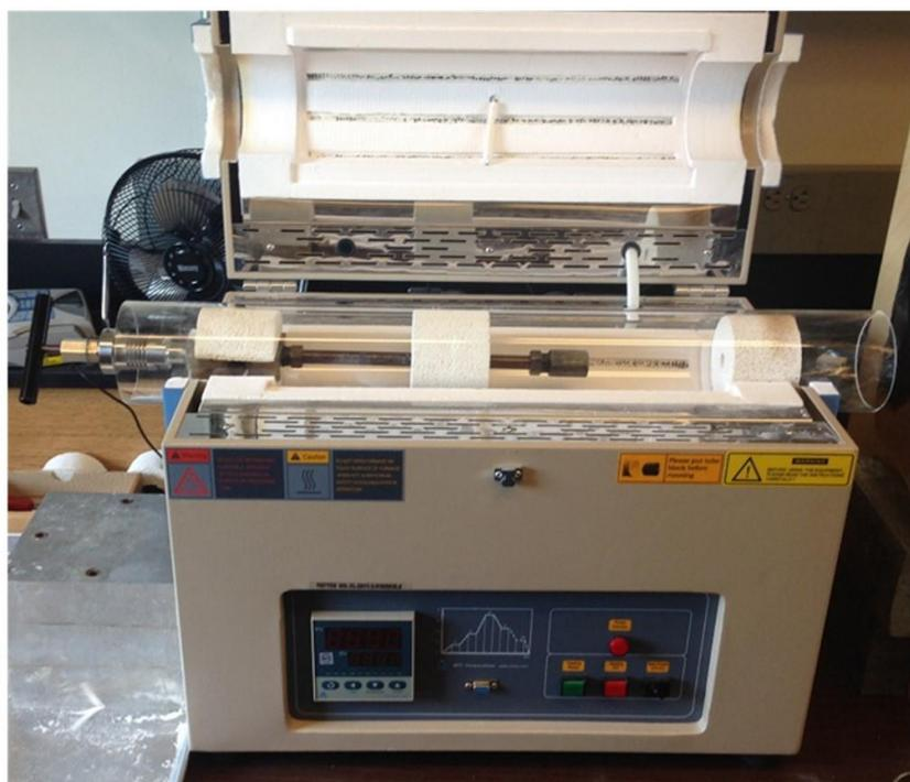
**Figure 1-1.** (Top) Metal tube reactor (MTR) schematic, (Bottom Left) Image of the assembled MTR, (Bottom Right) MTR set up inside the tube furnace. Firebricks were sculpted and cut to size to stabilize the MTR in the furnace ensuring even heating. A quartz tube was used to hold the firebricks and MTR in position inside the tube furnace.
