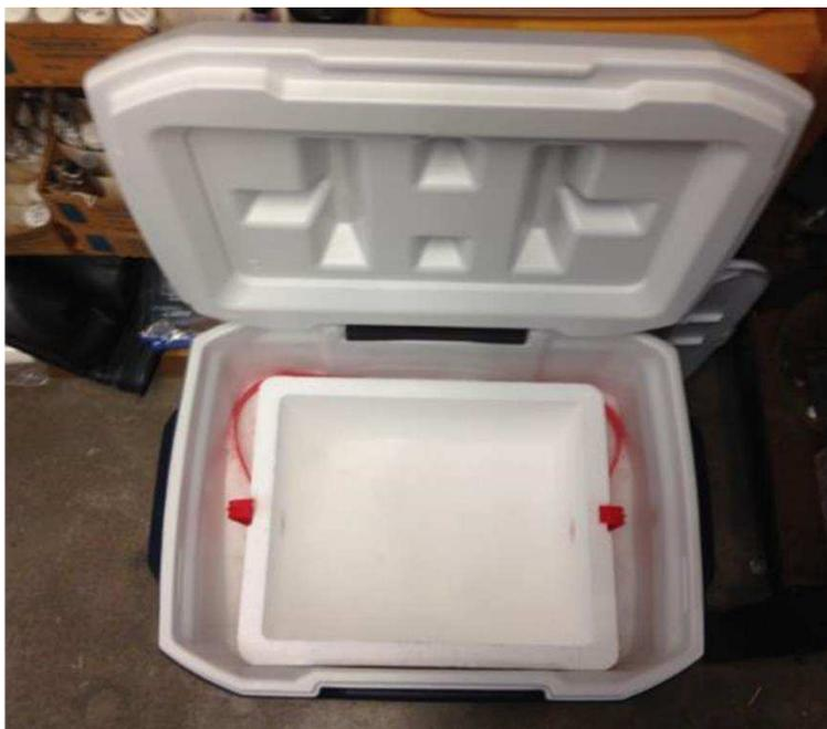
**Figure S4-1.** (Left) Air-tight vessel for thermal cycling of OPV active layers. The glass tube shows the arrangement of the slides inside the chamber. (Right) Low temperature chamber,  $-78\text{ }^{\circ}\text{C}$ . High temperature chamber,  $100\text{ }^{\circ}\text{C}$ , was a lab grade oven.
