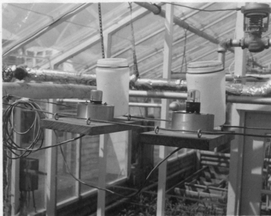
Figure 2.--Light sensing elements -- phototube (left) and solar battery (right).
