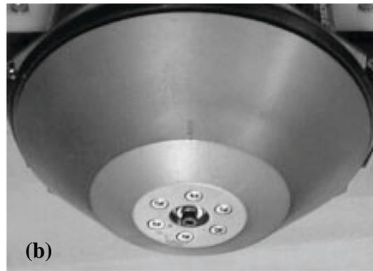
Reaction wheel for inertial steering
