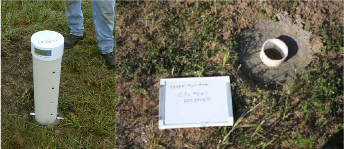
**Figure E.1.** CO<sub>2</sub> Trap housing and in-ground receiver. Note the green housing identification label on the trap housing (left). CO<sub>2</sub> Trap in-ground receiver as it appears when housing is removed (Right).
