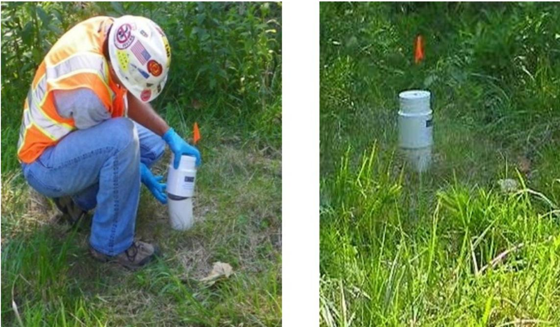
**Figure E.2.** CO<sub>2</sub> Trap installation. CO<sub>2</sub> Trap (left), note that white plastic field cap has been installed. CO<sub>2</sub> trap installed on receiver (right), note white plastic field cap.
