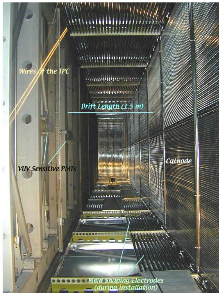
Figure 7.13: Inner mechanical structure of an ICARUS TPC module. Nine stainless steel panels make up the high-voltage cathode and can be seen on the right side of the image [64].
