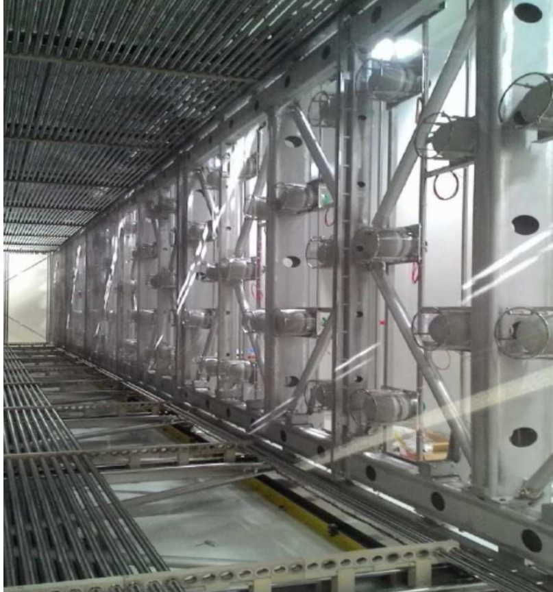
Figure 5.5: Mounted PMTs in an ICARUS TPC module. Photo from the ICARUS collaboration.
