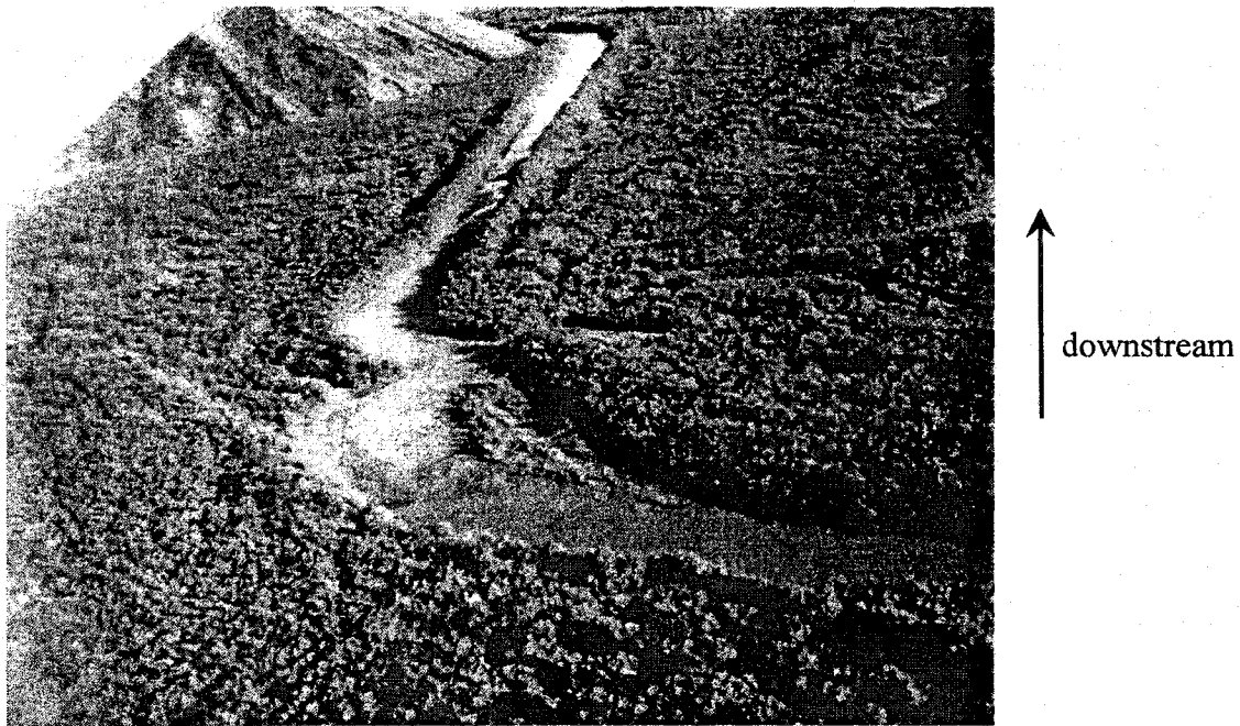
Figure 1.3 Sediment Plug that Initiated below Rangeline SO-1683 in 1991
