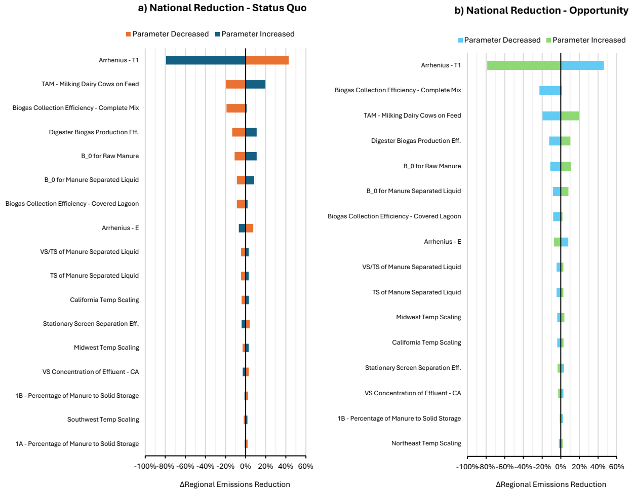
Figure B12: National Emissions Reduction Sensitivity Analysis Results for the Status Quo Case (a) and Opportunity Case (b). Input variables were adjusted by \pm 20\% and national emissions reduction potentials were recorded.
