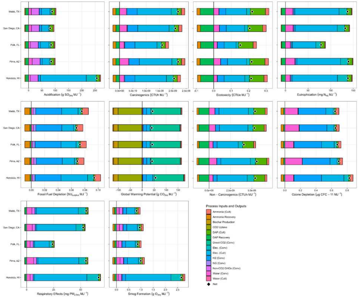
Figure A31: TRACI environmental impacts for renewable diesel production via HTL under the Future scenario. Results show the contribution of process consumables to each impact category for five case study locations including (from top to bottom) Webb County, Texas, San Diego County, California, Polk County, Florida, Pima County, Arizona, and Honolulu County, Hawaii.
