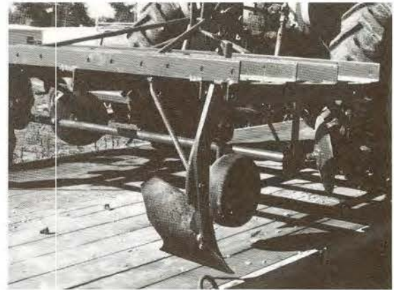
Machine for laying weed barrier. Slanted disks just behind the tractor wheels open a small furrow, barrier feeds from the bar behind the disks, the small, round wheels press the barrier into the furrow, and the plow turns a berm of soil over the barrier's edges. The machine is attached to the tractor with a 3-point hitch.
