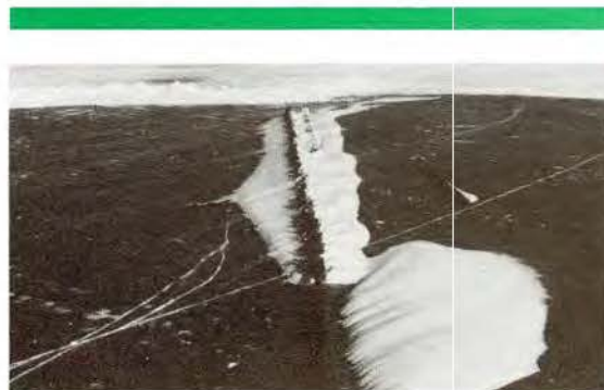
The barrier nearest the camera has a bottom gap while the other does not.
