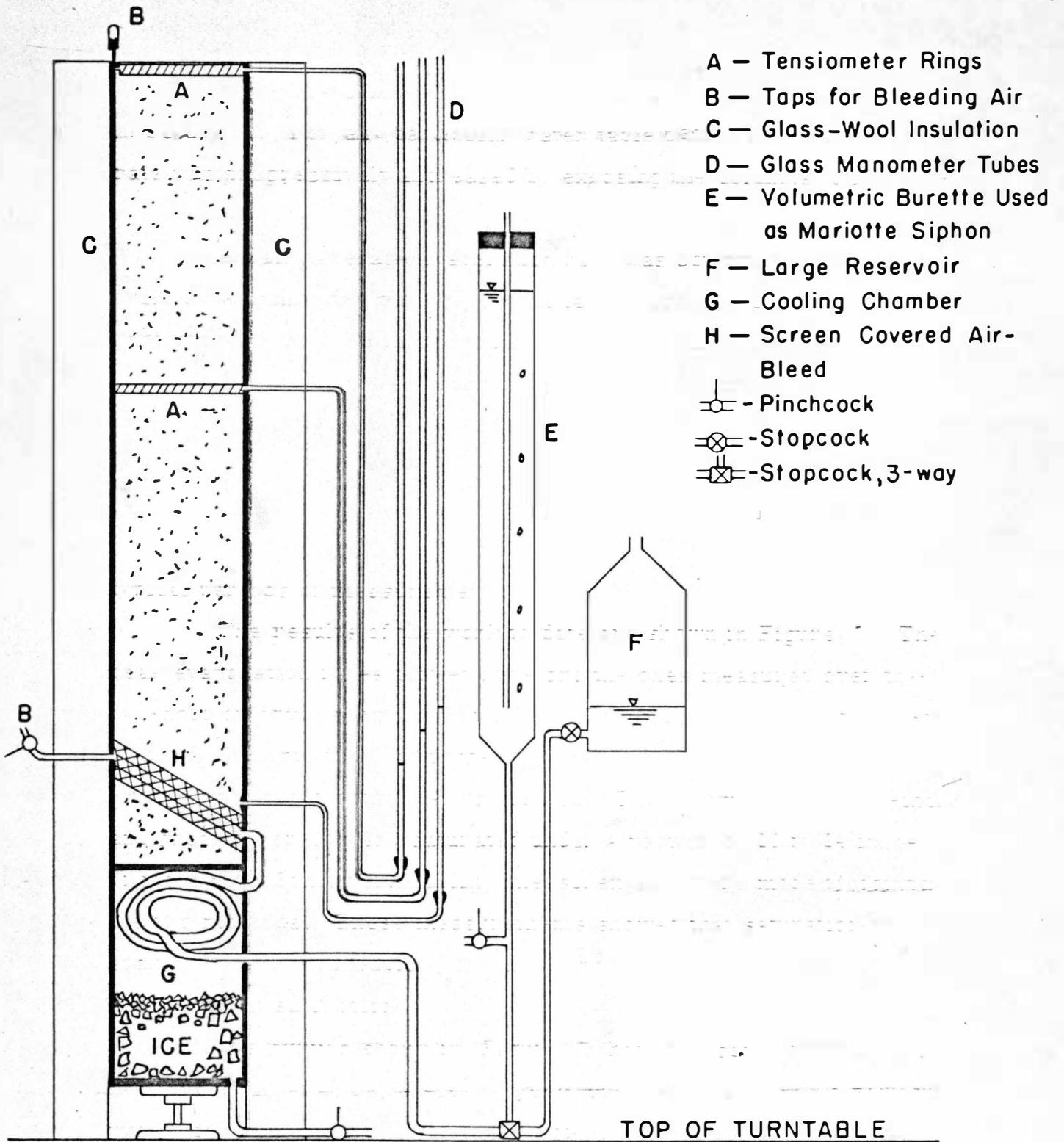
Fig. 5 Schematic Diagram of Evaporation Apparatus
