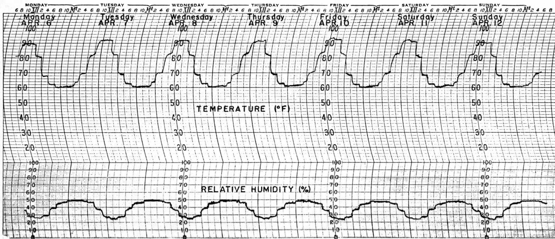
Fig. 4 Hygro-Thermograph Chart Showing Diurnal Cycles Produced in the Environmental Control Chamber
