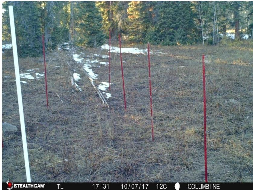
Figure A-2: Steel T posts used as snow staffs and as mounting points at sites without
