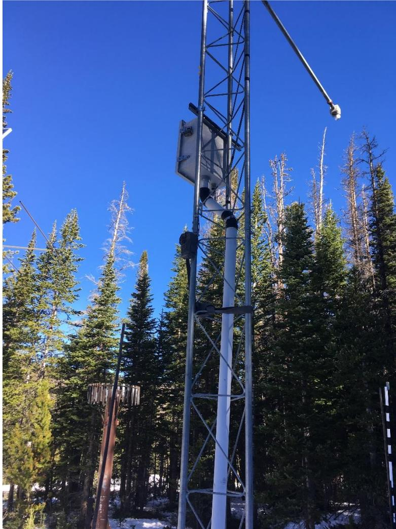
Figure A-3: Camera mounted on a SNOTEL meteorological tower at Joe Wright. A similar setup was used at Columbine and Red Mountain Pass
