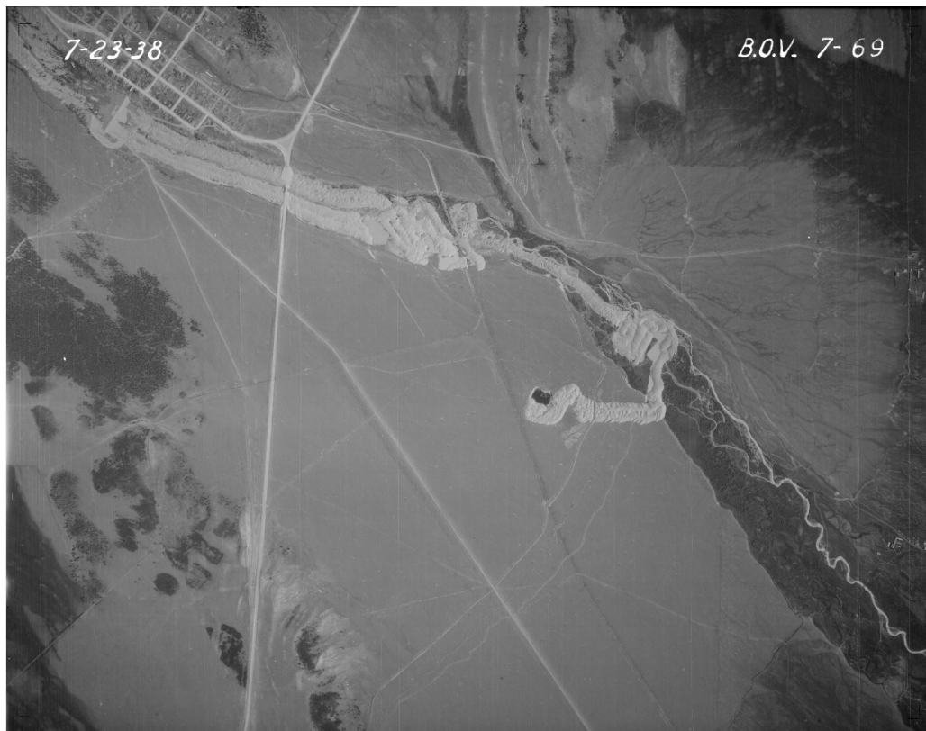
Figure 5. 1938 aerial photo of dredge mining near Fairplay, Colorado, in the South Platte Headwaters subbasin. Mining, as well as road construction, flood irrigation and other human activities were already occurring in the Project Area prior to the earliest aerial photos on record.
