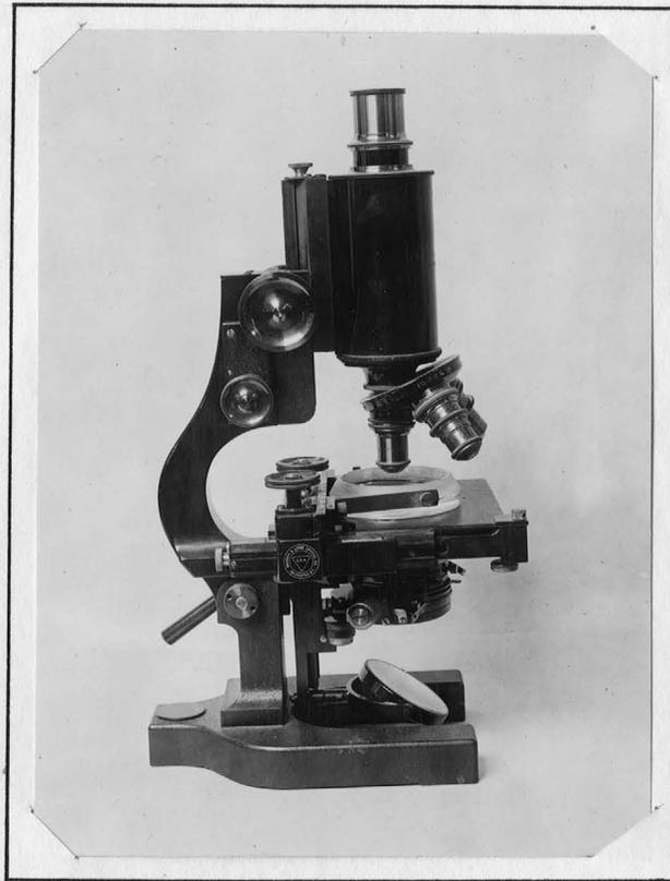
Fig. 4.- Microscope showing the Syracuse dish on the stage. The dish is readily moved by two screws at the left of the mechanical stage. A special clamp is screwed to the moving rack to hold the dish.
