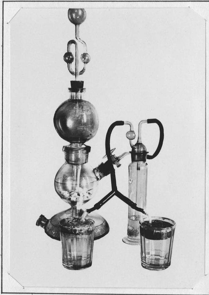
Fig. 6.- Apparatus for continuous bubbling of carbon dioxide into the spore suspensions.
