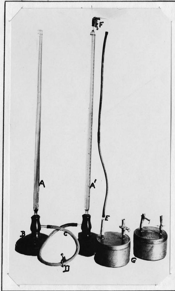
Fig. 5.- Gas burettes and two of the sealed culture chambers used in controlling the percentage of carbon dioxide in atmosphere of the spore suspensions.
