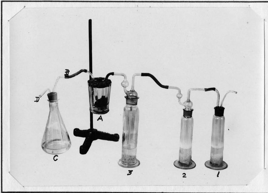
Fig. 7.- Apparatus used for determining the amount of carbon dioxide given off by a definite weight of plant tissue.
