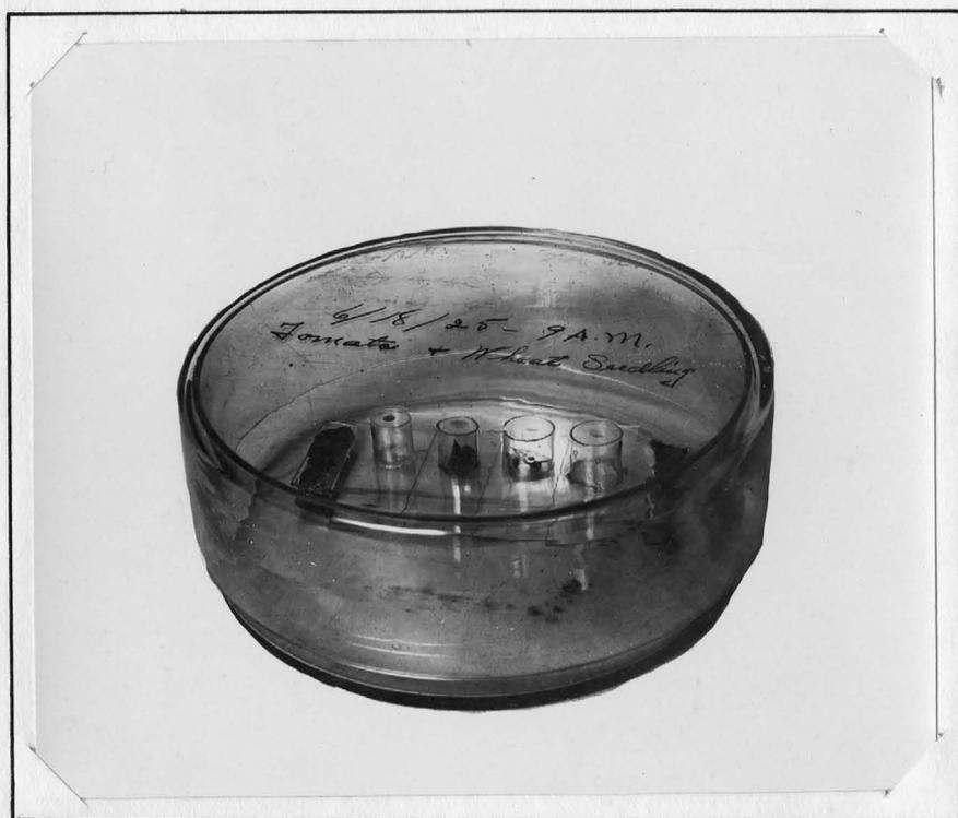
Fig. 2.- Showing arrangement of Van Tieghem cells in a moist chamber. The plant tissue is placed in the bottom of the cell with hanging drops of spore suspension on a cover glass over the cell. The cells are then placed on glass racks in moist chamber.
