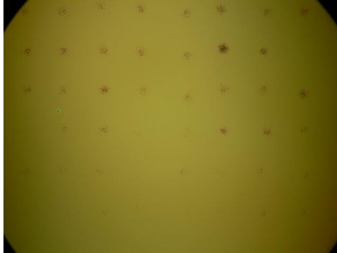
Figure 2.5) Nomarski microscope image at 5x magnification illustrating the result of a 1-on-1 LIDT test on an HfSiO x film. The high fluence rows are at the top, low fluence rows are at the bottom.
