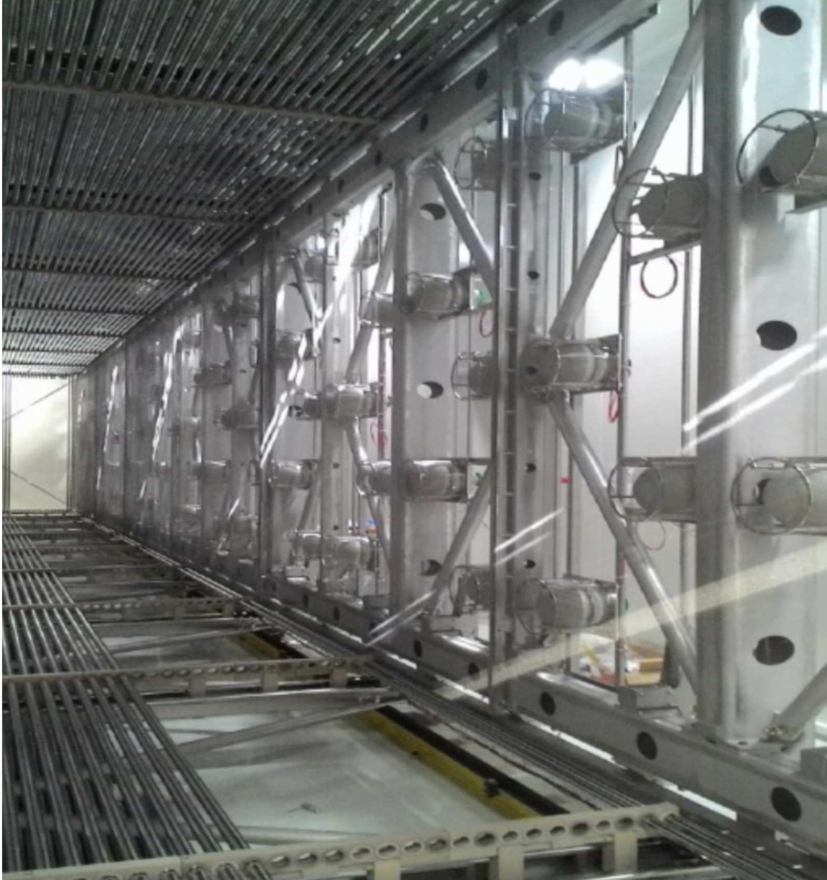
Figure 4.5: An image of the inside of one of the T300 submodules. The PMTs are visible mounted on the walls of the chamber behind the anode wire plane. The anode wire planes are only visible from the reflections glancing off the wires.
