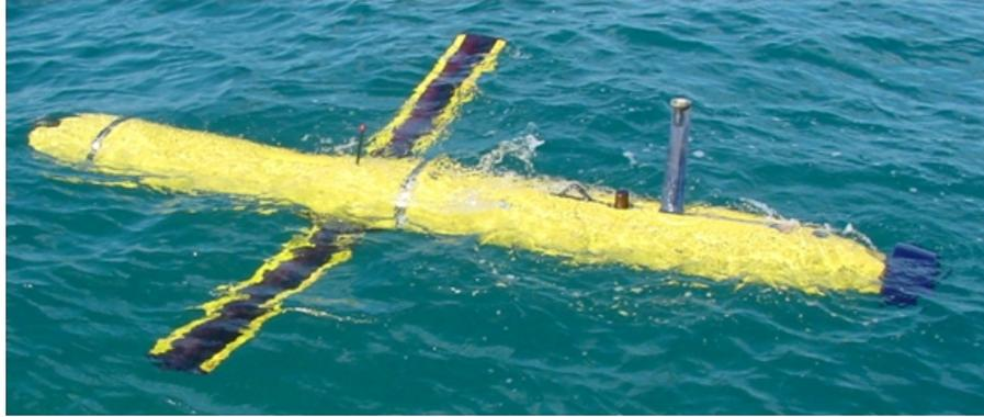
**Figure 3.7:** Bluefin 12 UUV with wing BOSS payload (courtesy of the FAU Department of Ocean Engineering).
