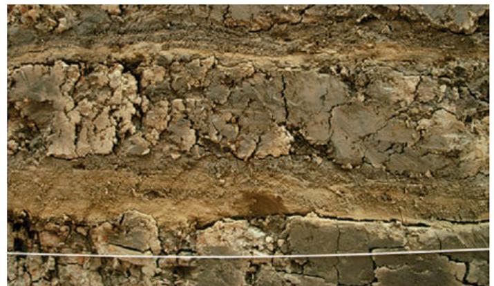
Figure 7. Layers in Morefield Canyon trench provide evidence of flooding history. Courtesy of Wright Paleohydrological Institute
