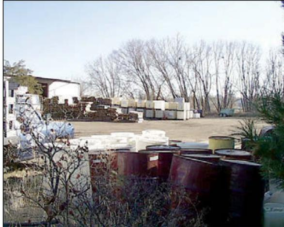
Figures 3 and 4. The Team Petroleum site on E. Lincoln Avenue is shown prior to clean-up of floatable materials. As part of the clean-up, all storage tanks were anchored to prevent them from floating away and all pallets, shipping containers and drums were either removed or secured inside a building.
