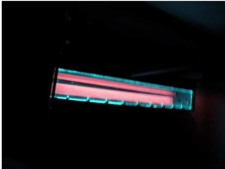
FIGURE 2.21. Trackway Lighting (Foreground: Green LED lit glass plate; Background: Red LED lit track enclosure)
