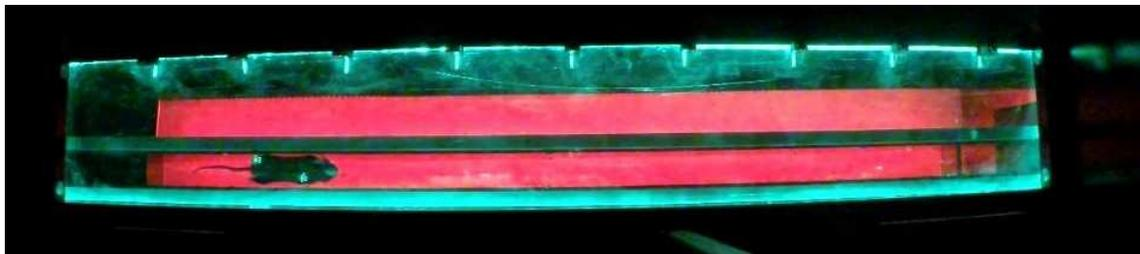
FIGURE 2.26. Original video frame with “barrel distortion”
