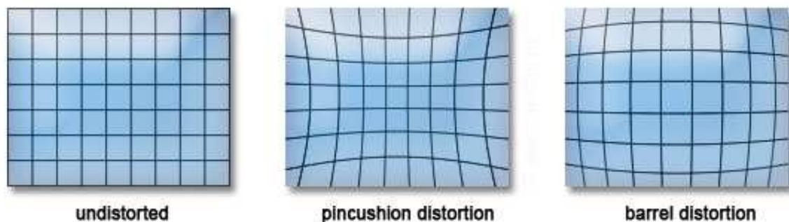
FIGURE 2.12. Types of Image Distortions (reprinted from [8])
