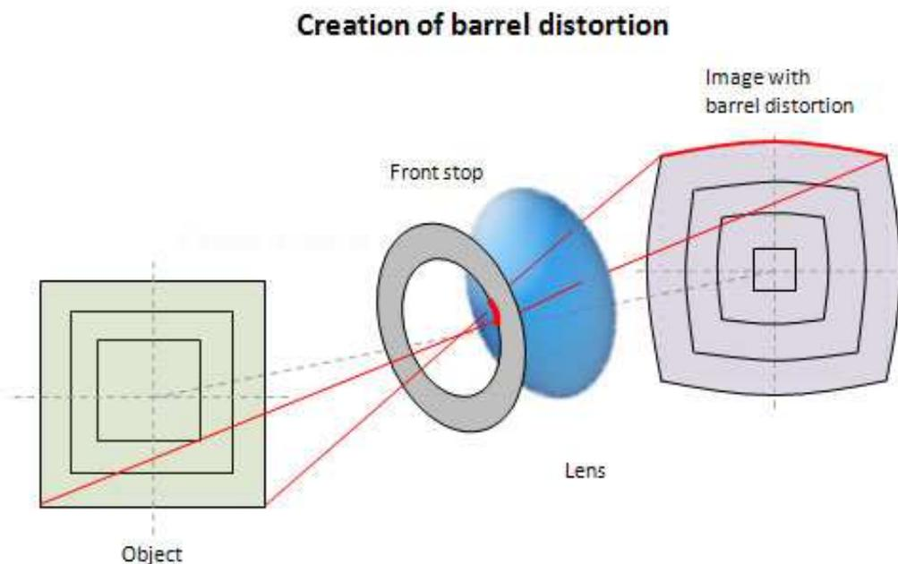
FIGURE 2.13. Creation of Barrel Distortion (reprinted from [8])
