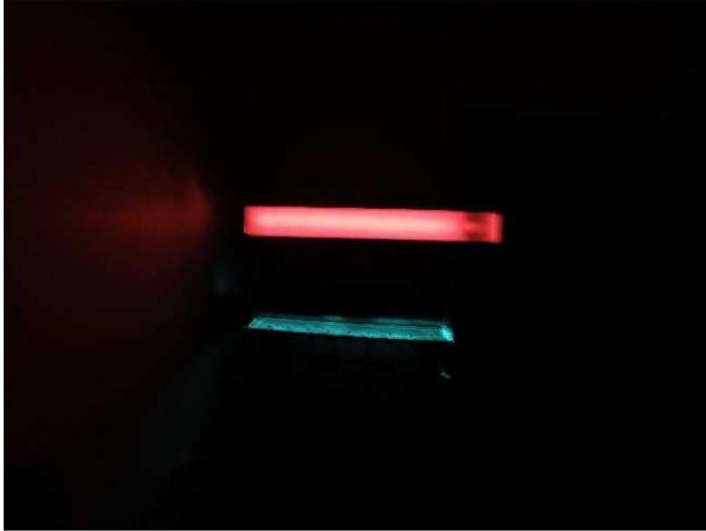
FIGURE 2.20. Trackway Lighting (Top: Red LED lit track enclosure; Bottom: Green LED lit glass plate)
