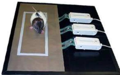
FIGURE 2.1. Tekscan Animal Walkway System (reprinted from [1])
