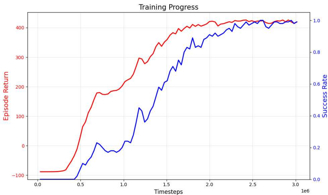
Figure 4.18: Training curves for the reaching task of the origami manipulator made of four modules. The episode return (blue, left axis) and success rate (red, right axis) are shown as functions of training timesteps. The agent achieves near-perfect success rate after 2.5 million timesteps.
