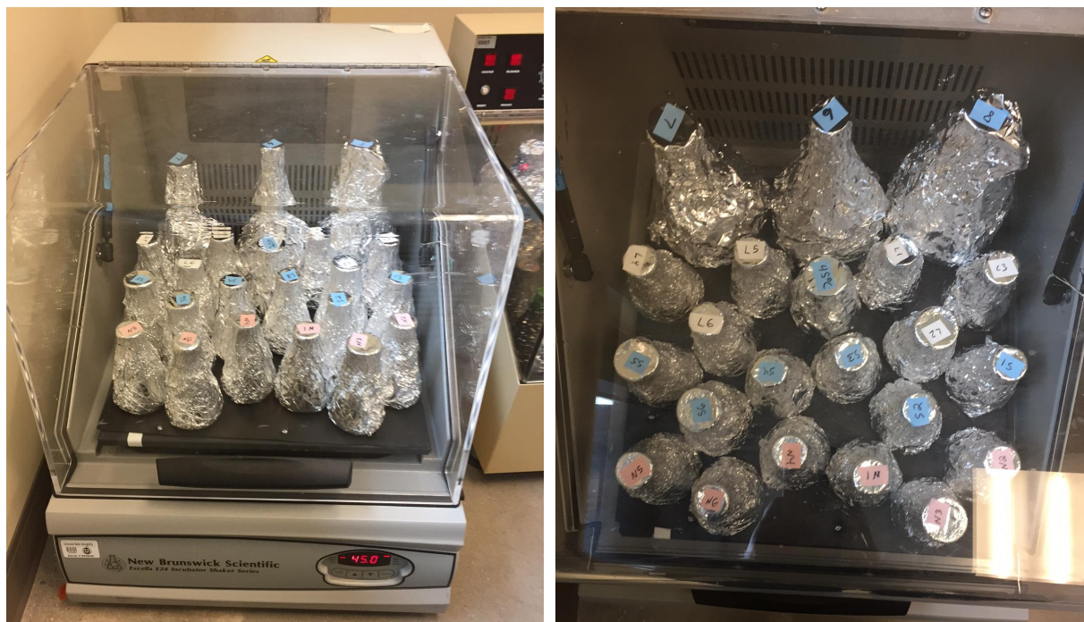
Figure 5: Photos of reactors in incubator shakers. All reactors were covered in foil, kept at constant temperature, and constantly shaken at 120 rpm.
